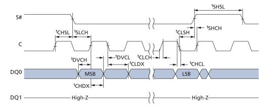
Figure 54: Write Protect Setup and Hold During WRITE STATUS REGISTER Operation (SRWD = 1)
