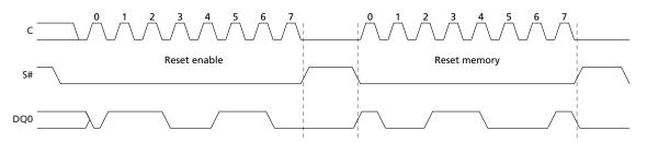
Figure 52: Serial Input Timing STR
