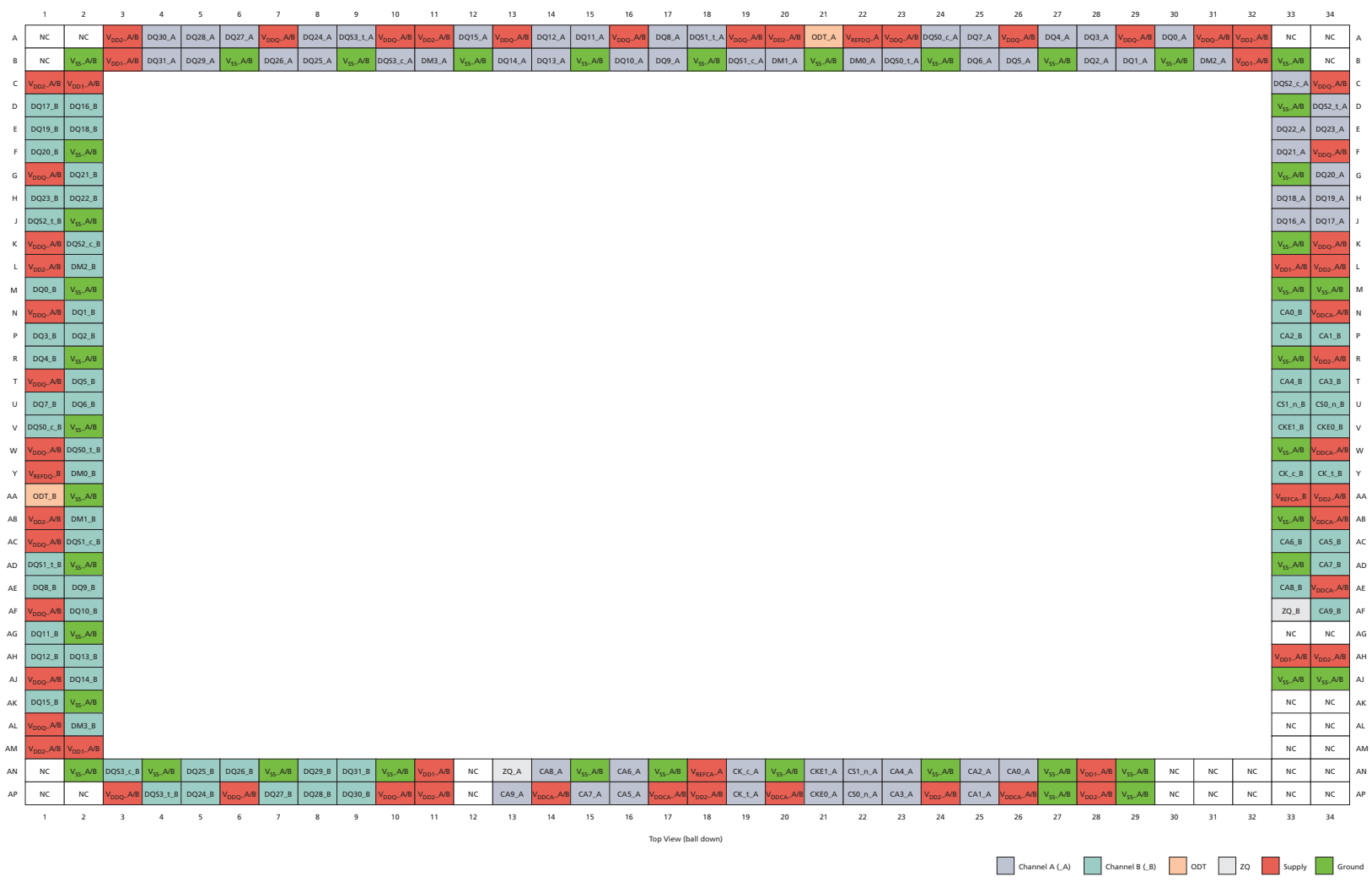
Figure 2: 256-Ball FBGA – 4 x 6Gb Die
