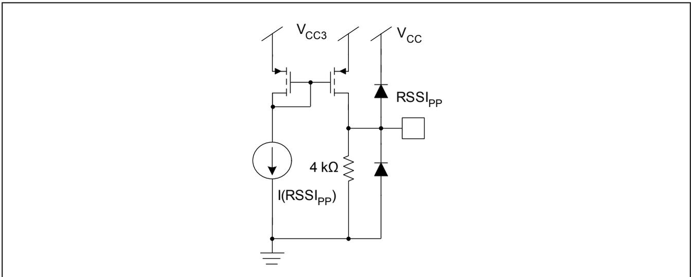
Figure 3-7. Typical  $RSSI_{pp}$  Transfer Function
