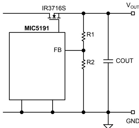
**Figure 10. Adjustable Output**
