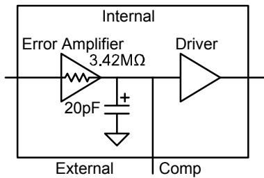
**Figure 3. Internal Compensation**
