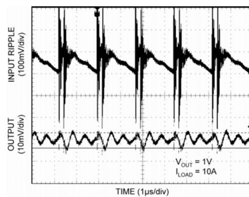
**Figure 11. Ripple Reduction**
