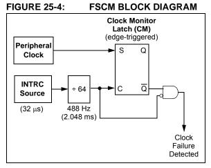
Clock failure is tested for on the falling edge of the sample clock. If a sample clock falling edge occurs while CM is still set, a clock failure has been detected (Figure 25-5). This causes the following:
