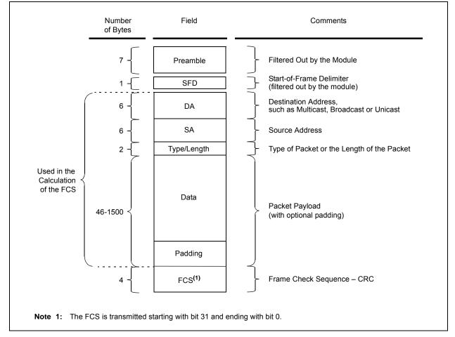
FIGURE 19-8: ETHERNET PACKET FORMAT
