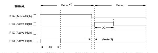
Note 1: The direction bit in the ECCP1 Control register (CCP1CON<7>) is written at any time during the PWM cycle.
