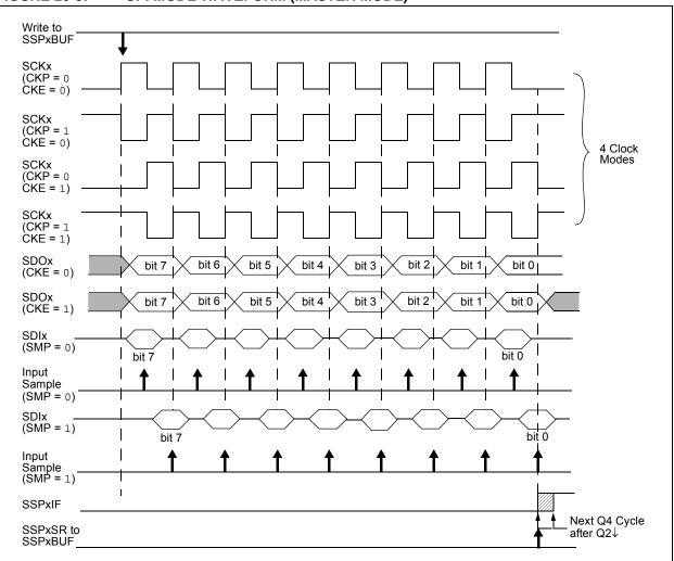
FIGURE 20-3: SPI MODE WAVEFORM (MASTER MODE)
