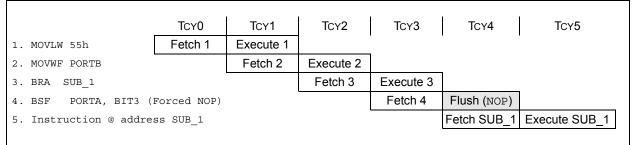
All instructions are single cycle, except for any program branches. These take two cycles since the fetch instruction is "flushed" from the pipeline while the new instruction is being fetched and then executed.
