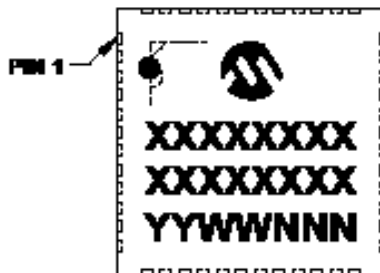
48-Lead UQFN (6x6x0.5 mm)
