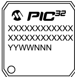
100-Lead TQFP (14x14x1 mm)
