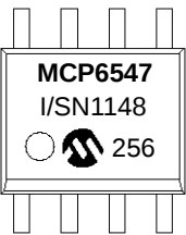
8-Lead SOIC (150 mil) (MCP6546, MCP6547, MCP6548, MCP6549)
