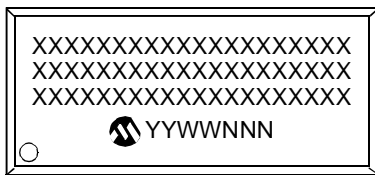
28-Lead SOIC (300 mil)
