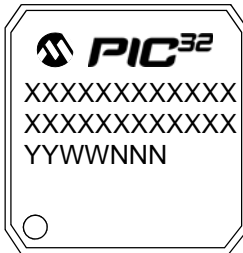
100-Lead TQFP (12x12x1 mm)
