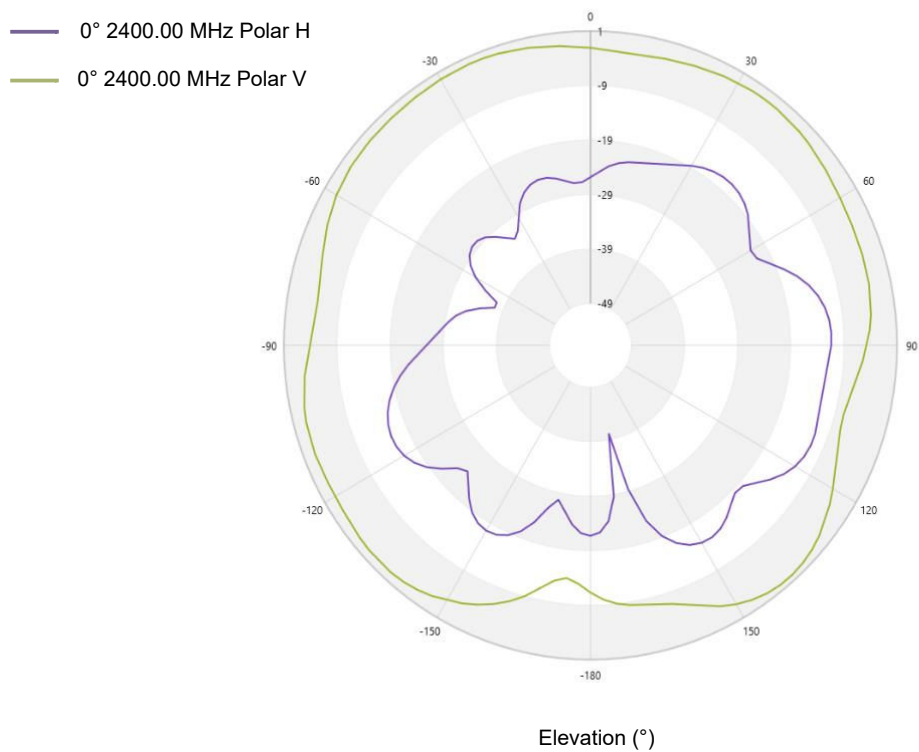
Figure 2-20. Antenna Radiation Elevated Plane Pattern @ \Phi = 90^\circ
