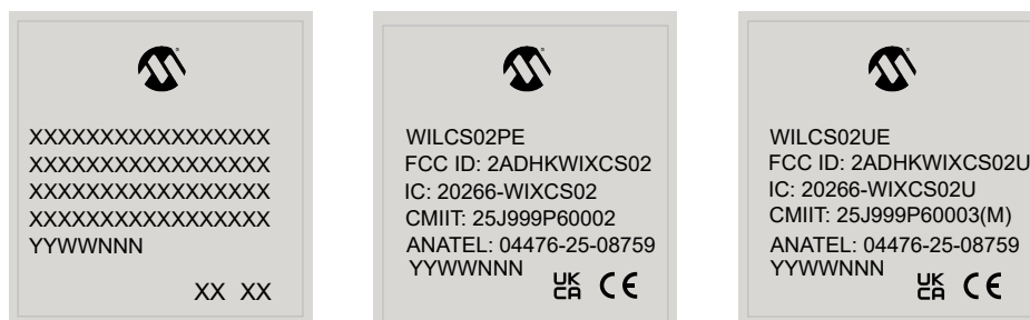
Figure 4-2. WILCS02 Module Packaging Marking
