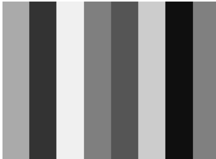
Figure 47.13. RGB888 BER Testing Pattern
