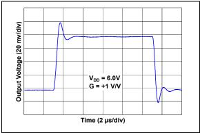
**FIGURE 2-29:** Small Signal Non-Inverting Pulse Response.
