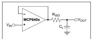
**FIGURE 4-4:** Output Resistor, R<sub>ISO</sub> Stabilizes Large Capacitive Loads.
