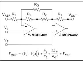
FIGURE 4-10: Two Op Amp Instrumentation Amplifier.
