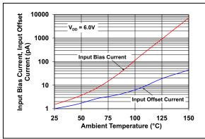
**FIGURE 2-15:** Input Bias, Offset Current vs. Ambient Temperature.
