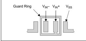
**FIGURE 4-7:** Example Guard Ring Layout for Inverting Gain.
