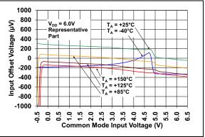
FIGURE 2-6: Input Offset Voltage vs. Common Mode Input Voltage with  $V_{DD} = 6.0V$ .
