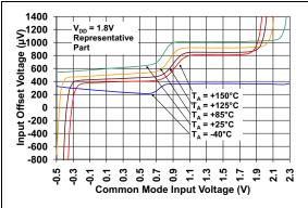
**FIGURE 2-7:** Input Offset Voltage vs. Common Mode Input Voltage with  $V_{DD} = 1.8V$ .
