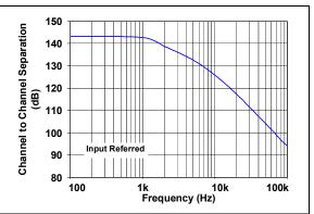
FIGURE 2-36: Channel-to-Channel Separation vs. Frequency (MCP6402/4/7/9 only).
