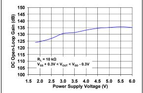
**FIGURE 2-20:** DC Open-Loop Gain vs. Power Supply Voltage.
