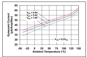
**FIGURE 2-17:** Quiescent Current vs. Ambient Temperature.
