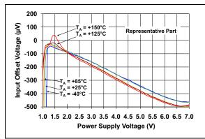
**FIGURE 2-9:** Input Offset Voltage vs. Power Supply Voltage.
