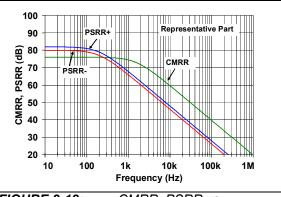
FIGURE 2-12: CMRR, PSRR vs. Frequency.
