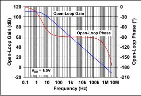
FIGURE 2-19: Open-Loop Gain, Phase vs. Frequency.
