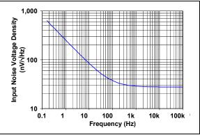
**FIGURE 2-10:** Input Noise Voltage Density vs. Frequency.
