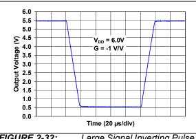
FIGURE 2-32: Large Signal Inverting Pulse Response.
