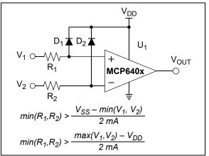
**FIGURE 4-3:** Protecting the Analog Inputs.
