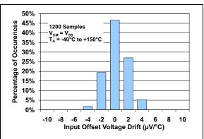
FIGURE 2-5: Input Offset Voltage Drift.
