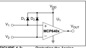
**FIGURE 4-2:** Protecting the Analog Inputs.
