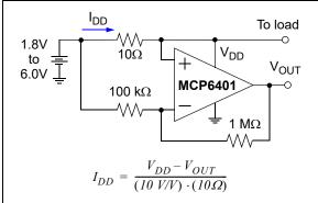
FIGURE 4-9: Supply Current Sensing.
