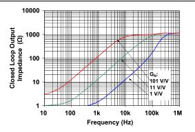
**FIGURE 2-34:** Closed Loop Output Impedance vs. Frequency.
