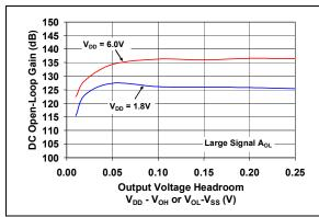
**FIGURE 2-21:** DC Open-Loop Gain vs. Output Voltage Headroom.
