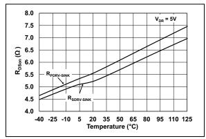
**FIGURE 7-11:** Sinking Output Driver  $R_{DSon}$  vs. Temperature.
