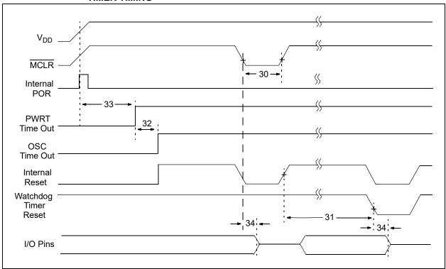
FIGURE 5-5: BROWN-OUT RESET TIMING AND CHARACTERISTICS
