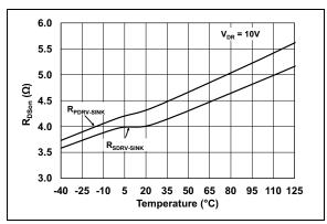
**FIGURE 7-9:** Sinking Output Driver  $R_{DSon}$  vs. Temperature.
