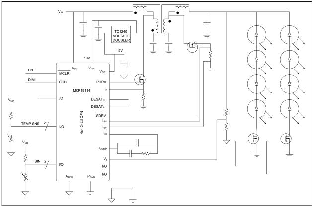
FIGURE 1-3: MCP19114 BOOST QUASI-RESONANT APPLICATION DIAGRAM
