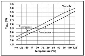
**FIGURE 7-10:** Sourcing Output Driver R<sub>DSon</sub> vs. Temperature.
