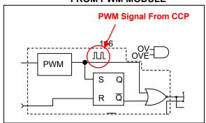
There are two modes of operation that concern the system clock PWM signal. These modes are Stand-Alone (nonfrequency synchronization) and Frequency Synchronization.
