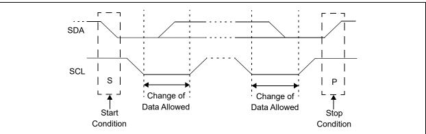
FIGURE 28-5: I<sup>2</sup>C RESTART CONDITION
