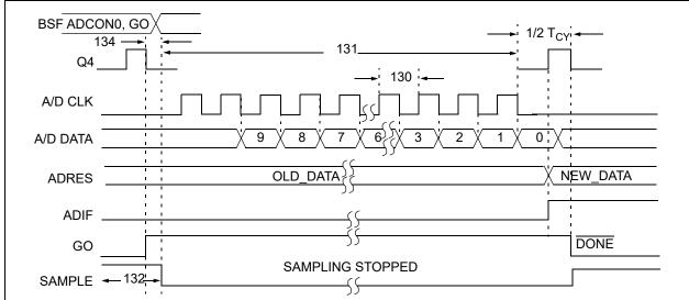
**Note 1:** If the A/D clock source is selected as RC, a time of  $T_{CY}$  is added before the A/D clock starts. This allows the SLEEP instruction to be executed.
