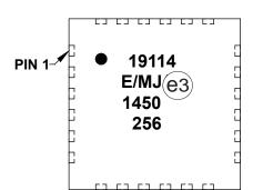
28-Lead QFN (5x5x0.9 mm)
