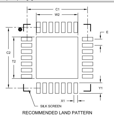
**MILLIMETERS** Units **Dimension Limits** MIN NOM MAX Contact Pitch Ε 0.50 BSC Optional Center Pad Width W2 3.35 Optional Center Pad Length T2 3.35 C1 4.90 Contact Pad Spacing Contact Pad Spacing C2 4.90 Contact Pad Width (X28) X1 0.30 Contact Pad Length (X28) 0.85
