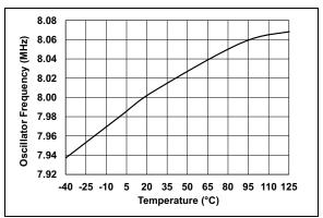
**FIGURE 7-12:** Oscillator Frequency vs. Temperature.
