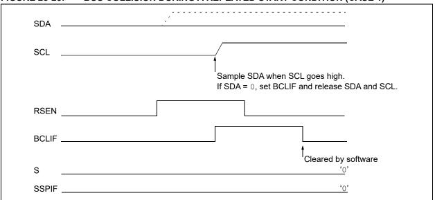
FIGURE 28-29: BUS COLLISION DURING A REPEATED START CONDITION (CASE 2)
