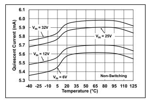
**FIGURE 7-1:**  $I_Q$  vs. Temperature.
