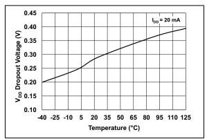
**FIGURE 7-6:** V<sub>DD</sub> Dropout Voltage vs. Temperature.
