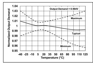
**FIGURE 7-13:** Normalized Output Demand vs. Temperature.
