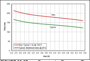
FIGURE 36-87: Comparator Response Time Falling edge, PIC16F18325/18345 Only
