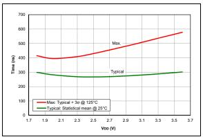
FIGURE 36-88: Comparator Response Time Rising edge, PIC16LF18325/18345 Only
