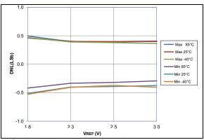
FIGURE 36-57: ADC 10-Bit Mode, Single-Ended DNL, VDD = 3.0V, TAD = 1 μs, All devices
