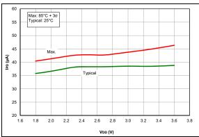
FIGURE 36-16: IPD, Fixed Voltage Reference (FVR), PIC16LF18325/18345 Only
