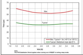
**FIGURE 36-91:** FVR Stabilization Period, PIC16LF18325/18345 Only
