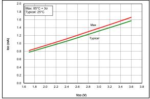
FIGURE 36-7: IDD, HFINTOSC Mode, Fosc = 16 MHz, PIC16LF18325/18345 Only
