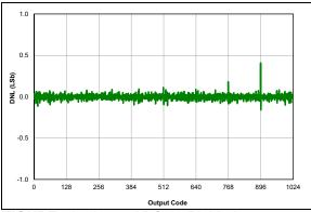
FIGURE 36-51: ADC 10-Bit Mode, Single-Ended DNL, VDD = 3.0V, VREF = 3.0V, TAD = 8 µs, 25°C, All devices
