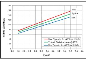
FIGURE 36-32: Weak Pull-Up Current, PIC16LF18325/18345 Only
