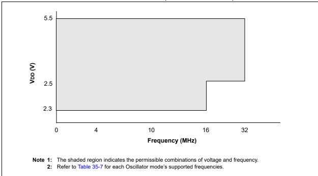
FIGURE 35-2: VOLTAGE FREQUENCY GRAPH, -40°C ≤TA ≤+125°C, PIC16LF18325/18345 ONLY
