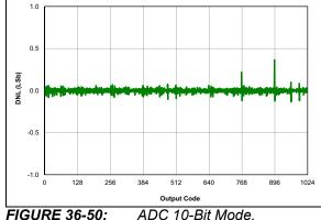
FIGURE 36-50: ADC 10-Bit Mode, Single-Ended DNL, VDD = 3.0V, VREF = 3.0V, TAD = 4 µs, 25°C, All devices
