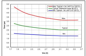
FIGURE 36-67: ADC RC Oscillator period, PIC16LF18325/18345 Only
