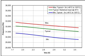
FIGURE 36-29: LFINTOSC Frequency, PIC16LF18325/18345 Only
