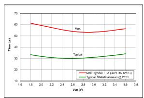
FIGURE 36-90: Band Gap Ready Time, PIC16LF18325/18345 Only
