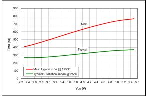
FIGURE 36-89: Comparator Response Time Rising edge, PIC16F18325/18345 Only
