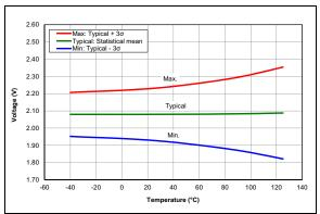
FIGURE 36-45: LPBOR Reset Voltage, PIC16LF18325/18345 only
