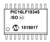
20-Lead SSOP (5.30 mm)
