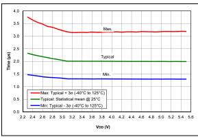
FIGURE 36-68: ADC RC Oscillator period, PIC16F18325/18345 Only
