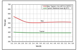
FIGURE 36-113: Wake From Sleep, VREGPM = 1, LFINTOSC, PIC16F18325/18345 Only
