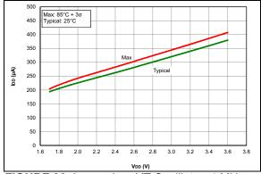
**FIGURE 36-1:** IDD, XT Oscillator, 4 MHz, PIC16LF18325/18345 Only
