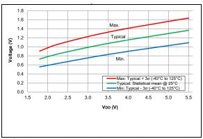
FIGURE 36-99: TTL Trip Thresholds, All devices
