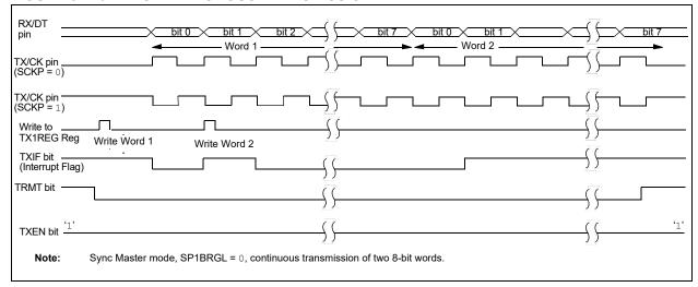
FIGURE 31-11: SYNCHRONOUS TRANSMISSION (THROUGH TXEN)
