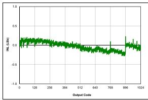
FIGURE 36-52: ADC 10-Bit Mode, Single-Ended INL, VDD = 3.0V, VREF = 3.0V, TAD = 1 µs, 25°C, All devices
