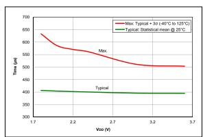
FIGURE 36-114: Wake From Sleep, LFINTOSC, PIC16LF18325/18345 Only
