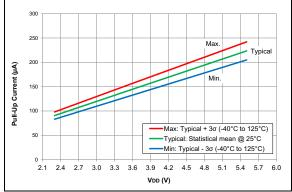
FIGURE 36-31: Weak Pull-Up Current, PIC16F18325/18345 Only
