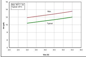
**FIGURE 36-19:** IPD, Brown-out Reset (BOR), BORV = 1, PIC16F18325/18345 Only
