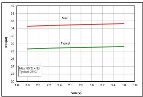
**FIGURE 36-22:** IPD, Comparator, PIC16LF18325/18345 Only
