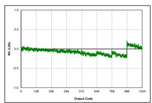
FIGURE 36-54: ADC 10-Bit Mode, Single-Ended INL, VDD = 3.0V, VREF = 3.0V, TAD = 8 μs, 25°C, All devices
