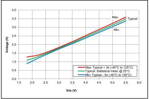
FIGURE 36-97: Schmitt Trigger High Values, All devices
