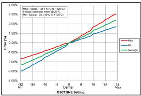
FIGURE 36-104: OSCTUNE Center Frequency, PIC16LF18325/18345 Only
