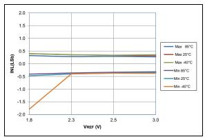
FIGURE 36-58: ADC 10-Bit Mode, Single-Ended INL, VDD = 3.0V, TAD = 1 μs, All devices
