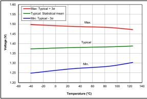
FIGURE 36-105: POR Release Voltage, All devices
