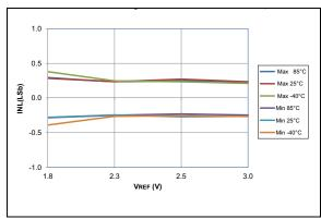
FIGURE 36-62: ADC 10-Bit Mode, Single-Ended INL, VDD = 3.0V, TAD = 4 μs, All devices
