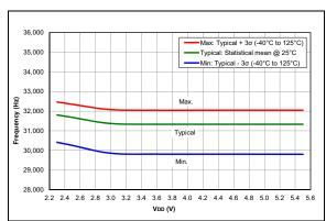
FIGURE 36-30: LFINTOSC Frequency, PIC16F18325/18345 Only
