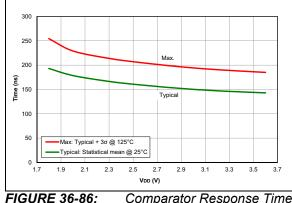
FIGURE 36-86: Comparator Response Time Falling edge, PIC16LF18325/18345 Only
