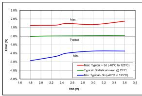
FIGURE 36-26: HFINTOSC Typical Frequency Error, PIC16LF18325/18345 Only
