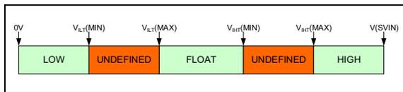
**FIGURE 4-3:** SELVx High, Low and Float States Threshold.
