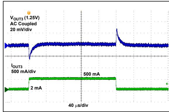
**FIGURE 2-18:** Buck3 Transient Response (Active Mode,  $V_{OUT3} = 1.25V$ ).
