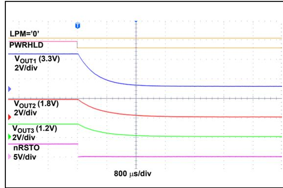
**FIGURE 2-16:** PWRHLD Shutdown Sequence.
