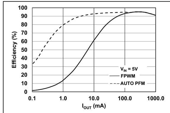
**FIGURE 2-4:** Buck1 Efficiency vs. Load Current ( $V_{OUT1} = 3.3V$ ).
