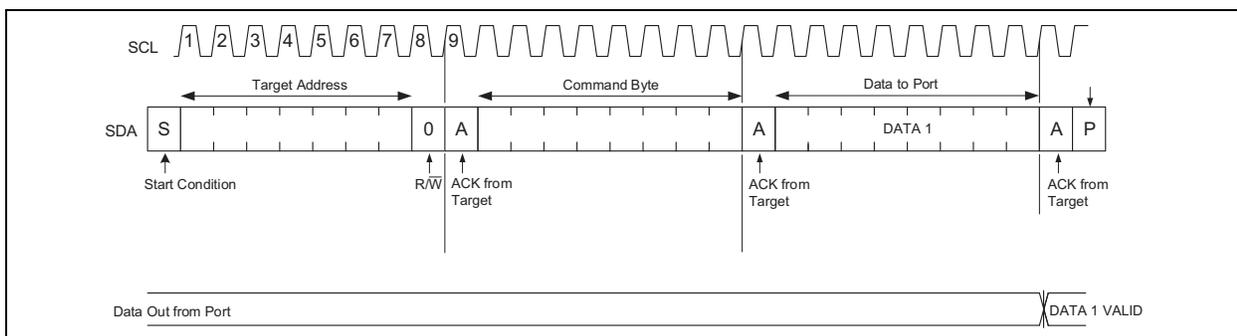
FIGURE 4-12: I<sup>2</sup>C Single Write.
