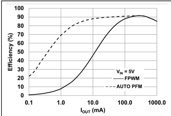
**FIGURE 2-7:** Buck4 Efficiency vs. Load Current ( $V_{OUT3} = 1.8V$ ).
