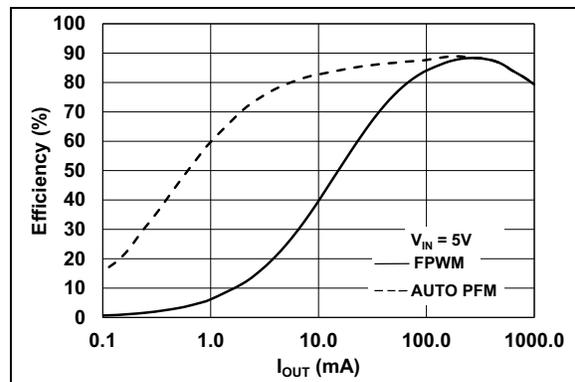
**FIGURE 2-5:** Buck2 Efficiency vs. Load Current ( $V_{OUT2} = 1.2V$ ).
