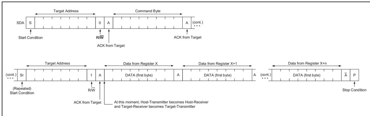
**FIGURE 4-15:** I<sup>2</sup>C Block Read.
