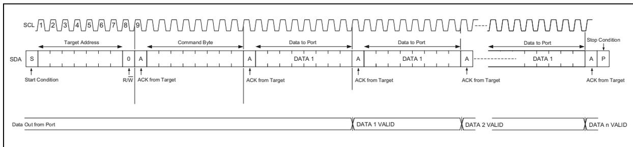
**FIGURE 4-13:** Block Write.
