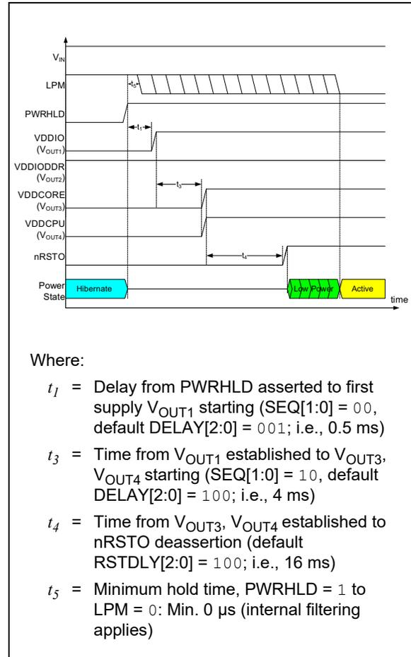
**FIGURE 4-10:** Start-Up Sequence Exiting Hibernate Mode Timing Diagram.
