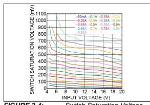
FIGURE 2-4: Switch Saturation Voltage vs. Input Voltage.
