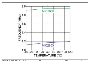
FIGURE 2-15: Frequency vs. Temperature.
