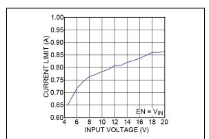
FIGURE 2-6: Switch Current Limit vs. Input Voltage.
