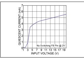
FIGURE 2-2: Quiescent Current vs. Input Voltage.
