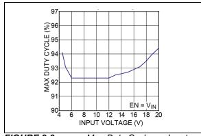
FIGURE 2-3: Max Duty Cycle vs. Input Voltage.
