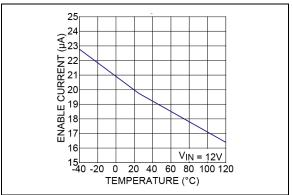
FIGURE 2-16: Enable Current vs. Temperature.
