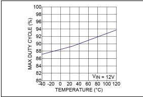
FIGURE 2-14: Max Duty Cycle vs. Temperature.
