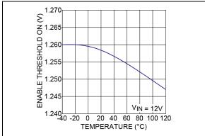
**FIGURE 2-13:** Enable Threshold Voltage  $(V_{EN})$  vs. Temperature.
