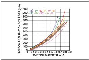
FIGURE 2-5: Switch Saturation Voltage vs. Switch Current.
