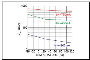
**FIGURE 2-12:** Switch Saturation Voltage  $(V_{SW})$  vs. Temperature.
