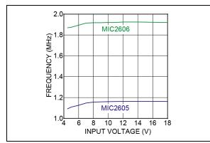
FIGURE 2-1: Frequency vs. Input Voltage.
