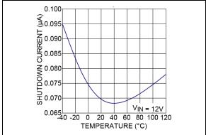
FIGURE 2-17: Shutdown Current vs. Temperature.
