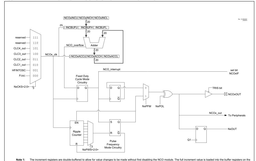
second rising edge of the NCOx\_clk signal that occurs immediately after a write to NCOxINCL register. The buffers are not user-accessible and are shown here for reference.
