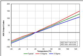
FIGURE 38-49: Temp. Indicator Slope Normalized to 20°C, Low Range, VDD = 2.3V.
