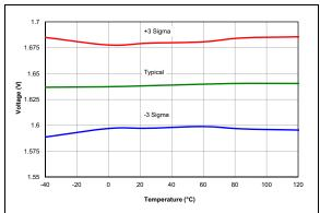
FIGURE 38-23: POR Release Voltage.
