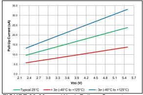
FIGURE 38-89: Weak Pull-up Current, PIC16F18857/77 Only.
