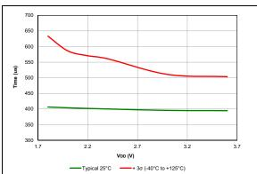
FIGURE 38-32: Wake From Sleep, LFINTOSC, PIC16LF18857/77 Only.
