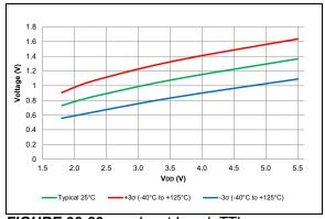
FIGURE 38-83: Input Level, TTL.
