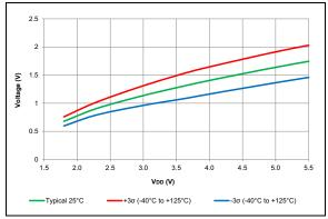
FIGURE 38-82: Schmitt Trigger Low Values.
