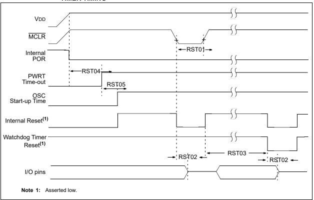
FIGURE 37-9: BROWN-OUT RESET TIMING AND CHARACTERISTICS
