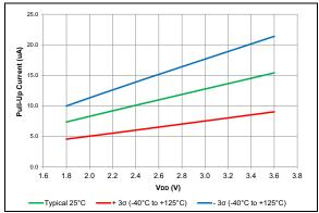
FIGURE 38-90: Weak Pull-up Current, PIC16LF18857/77 Only.
