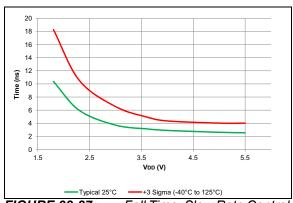
**FIGURE 38-87:** Fall Time, Slew Rate Control Disabled.
