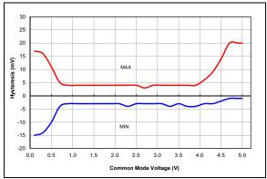
FIGURE 38-54: Comparator Offset, NP Mode (CxSP = 1), VDD = 5.0V, Typical Measured Values at 25°C, PIC16F18857/77 Only.
