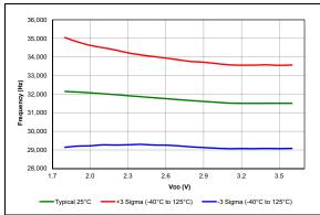
FIGURE 38-7: LFINTOSC Frequency, PIC16LF18857/77 Only.
