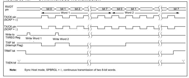
FIGURE 33-11: SYNCHRONOUS TRANSMISSION (THROUGH TXEN)
