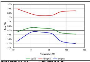
FIGURE 38-80: HFINTOSC Frequency Error, VDD = 3.0V.
