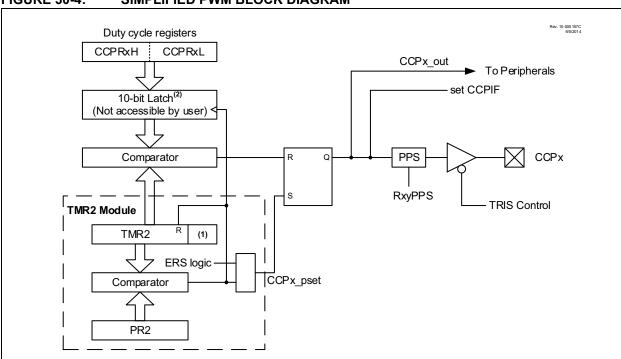
FIGURE 30-4: SIMPLIFIED PWM BLOCK DIAGRAM
