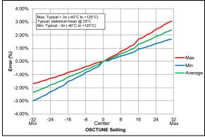
FIGURE 38-88: OSCTUNE Center Frequency, PIC16LF18857/77 Only.
