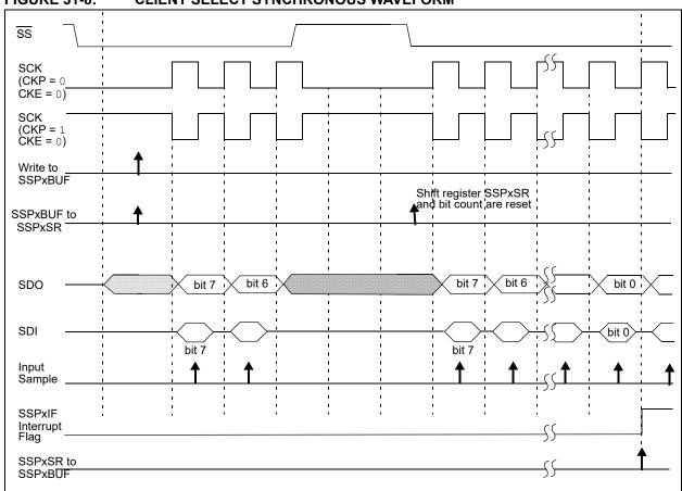
FIGURE 31-9: SPI MODE WAVEFORM (CLIENT MODE WITH CKE = 0)
