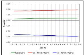
FIGURE 38-79: HFINTOSC Typical Frequency Error, PIC16F18857/77 Only.
