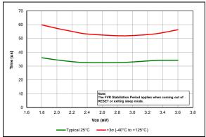
FIGURE 38-72: FVR Stabilization Period, PIC16LF18857/77 Only.
