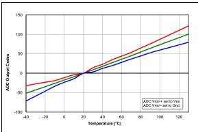
FIGURE 38-48: Temp. Indicator Slope
