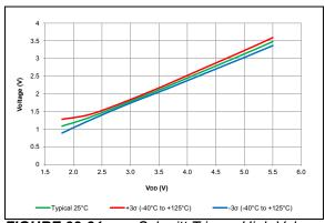
FIGURE 38-81: Schmitt Trigger High Values.
