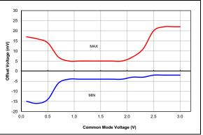
FIGURE 38-52: Comparator Offset, NP Mode (CxSP = 1), VDD = 3.0V, Typical Measured Values from -40°C to 125°C.
