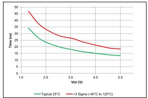
FIGURE 38-84: Rise Time, Slew Rate Control Enabled.
