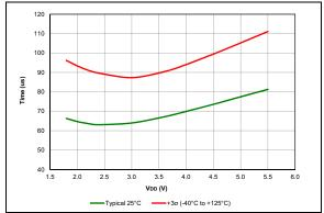
FIGURE 38-30: Wake From Sleep, VREGPM = 1, HFINTOSC = 16 MHz, PIC16F18857/77 Only.
