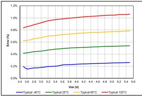
**FIGURE 38-74:** FVR Voltage Error 1x, PIC16F18857/77 Only.
