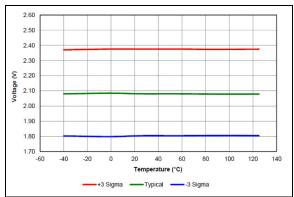
**FIGURE 38-19:** LPBOR Reset Voltage, PIC16LF18857/77 Only.
