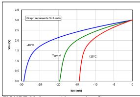
FIGURE 38-3: VOH vs. IOH Over Temperature, VDD = 3.0V.
