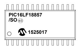
28-Lead SSOP (5.30 mm)
