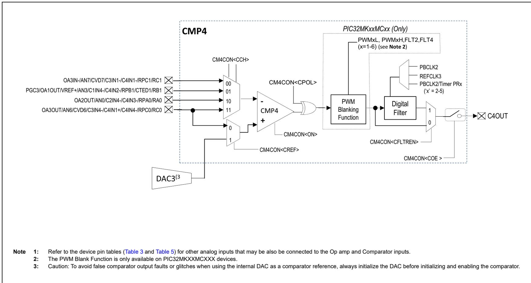
FIGURE 27-5: OP AMP 5/COMPARATOR 5 MODULE BLOCK DIAGRAM
