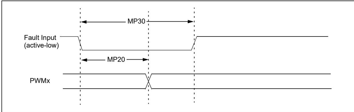
**TABLE 37-51: MOTOR CONTROL PWM MODULE TIMING REQUIREMENTS**
