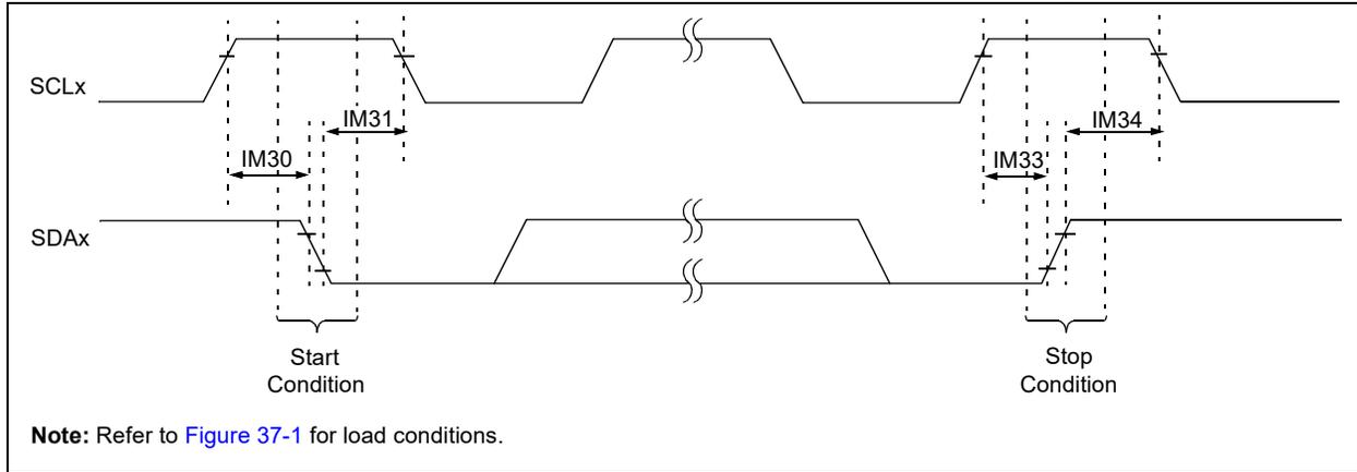
**FIGURE 37-15: I2Cx BUS DATA TIMING CHARACTERISTICS (MASTER MODE)**
