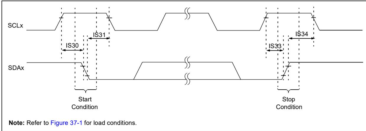
**FIGURE 37-17: I2Cx BUS DATA TIMING CHARACTERISTICS (SLAVE MODE)**
