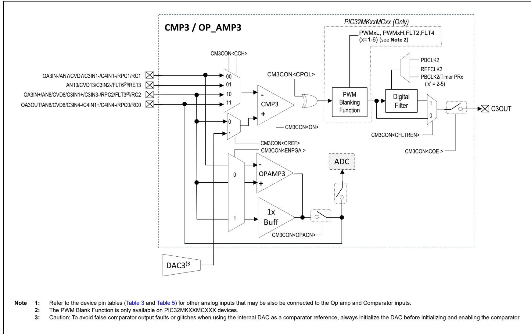
FIGURE 27-4: COMPARATOR 4 MODULE BLOCK DIAGRAM
