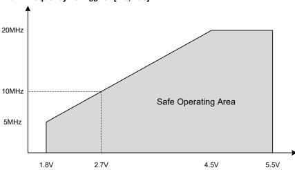
Figure 32-1. Maximum Frequency vs. V<sub>DD</sub> for [-40, 105]°C
