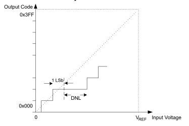
**Quantization Error** Due to the quantization of the input voltage into a finite number of codes, a range of input
