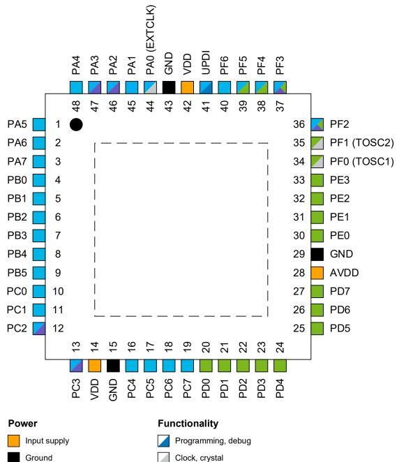
**Note:** The center pad underneath the QFN packages can be connected to PCB ground or left electrically unconnected. Solder or glue it to the board to ensure good mechanical stability. If the center pad is not attached, the package might loosen from the board.
