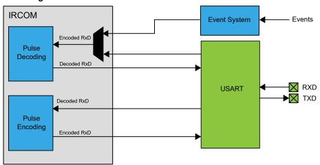
The USART is set in IRCOM mode by writing 0x02 to the CMODE bits in the USARTn.CTRLC register. The data on the TXD/RXD pins are the inverted values of the transmitted/received infrared pulse. It is also possible to select an event channel from the Event System as an input for the IRCOM receiver. This enables the IRCOM to receive input from the I/O pins or sources other than the corresponding RXD pin. This will disable the RxD input from the USART pin.
