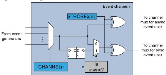
The block diagram shows the operation of an event channel. A multiplexer controlled by EVSYS.CHANNELn at the input selects which of the event sources to route onto the event channel. Each event channel has two subchannels; One asynchronous subchannel and one synchronous subchannel. A synchronous user will listen to the synchronous subchannel, an asynchronous user will listen to the asynchronous subchannel.
