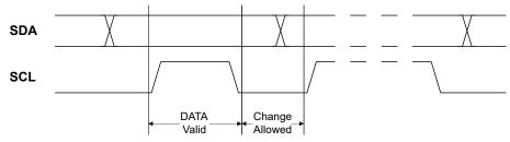
Combining bit transfers result in the formation of address and data packets. These packets consist of eight data bits (one byte) with the Most Significant bit transferred first, plus a single-bit not-Acknowledge (NACK) or Acknowledge (ACK) response. The addressed device signals ACK by pulling the SCL line low during the ninth clock cycle, and signals NACK by leaving the line SCL high.
