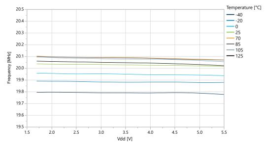
Figure 33-71. OSC20M Internal Oscillator: Frequency vs. V<sub>DD</sub>
