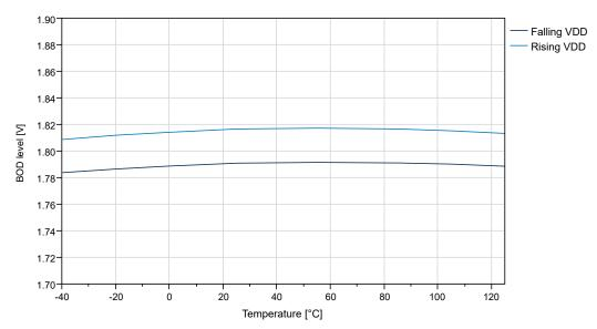
Figure 33-42. BOD Threshold vs. Temperature (BODLEVEL2)
