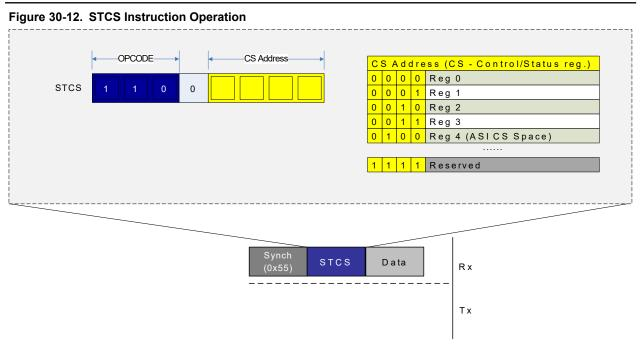
Figure 30-12 shows the data frame transmitted after the SYNCH and instruction frames. There is no response generated from the STCS instruction, as is the case for ST and STS.
