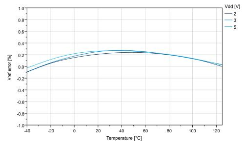
Figure 33-36. Internal 2.5V Reference vs. Temperature
