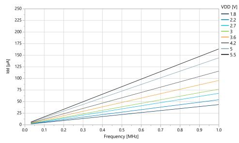
Figure 33-9. Idle Supply Current vs. Low Frequency (0.1-1.0 MHz) at T = 25 °C
