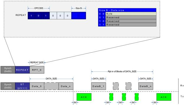
The figure above gives an example of repeat operation with an ST instruction using pointer post-increment operation. After the REPEAT instruction is sent with RPT\_0 =  $\mathbf{n}$ , the first ST instruction is issued with SYNCH and Instruction frame, while the next  $\mathbf{n}$  ST instructions are executed by only sending in data bytes according to the ST operand DATA SIZE, and maintaining the Acknowledge (ACK) handshake protocol.
