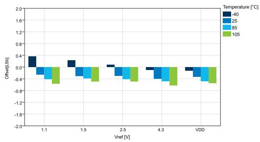
Figure 33-53. Offset Error vs.  $V_{REF}$  ( $V_{DD}$  = 5.0V,  $f_{ADC}$  = 115 ksps), REFSEL = Internal Reference
