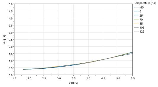
Figure 33-40. BOD Current vs. V<sub>DD</sub> (Sampled BOD at 1 kHz)
