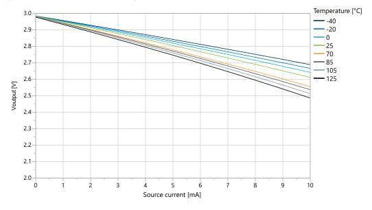
Figure 33-29. I/O Pin Output Voltage vs. Source Current ( $V_{DD} = 5.0V$ )
