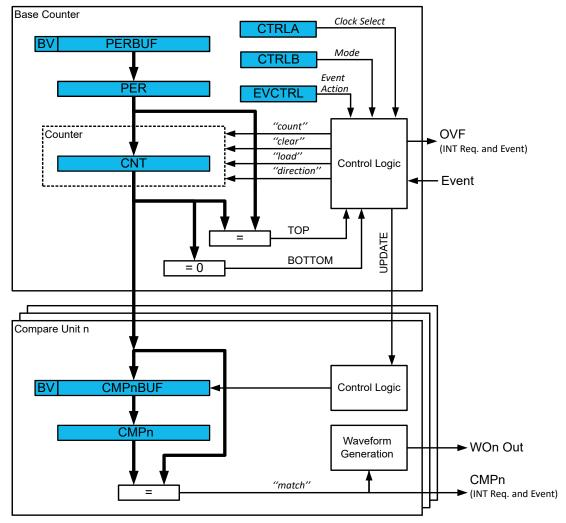
The Counter register (TCAn.CNT), Period and Compare registers (TCAn.PER and TCAn.CMPm) and their corresponding buffer registers (TCAn.PERBUF and TCAn.CMPBUFm) are 16-bit registers. All buffer registers have a Buffer Valid (BV) flag that indicates when the buffer contains a new value.
