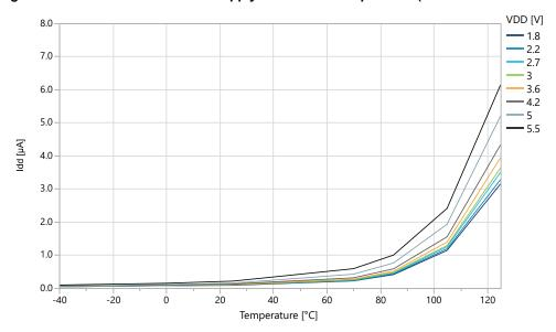
Figure 33-14. Power-Down Mode Supply Current vs.  $V_{DD}$  (all functions disabled)
