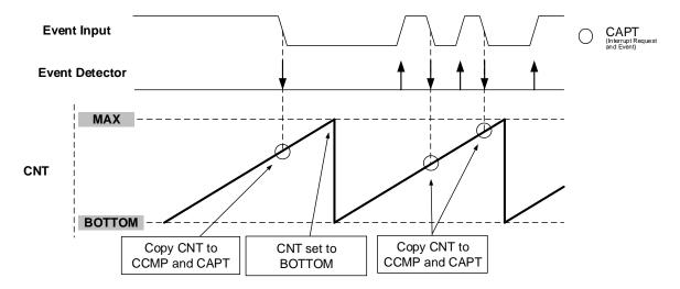
It is recommended to write zero to the TCBn.CNT register when entering this mode from any other mode.
