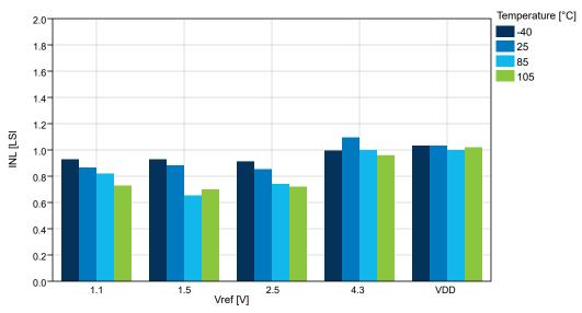
Figure 33-51. INL vs.  $V_{REF}$  ( $V_{DD}$  = 5.0V,  $f_{ADC}$  = 115 ksps), REFSEL = Internal Reference
