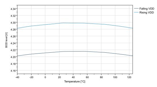
Figure 33-43. BOD Threshold vs. Temperature (BODLEVEL7)
