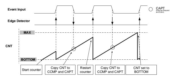
Figure 21-7. Input Capture Pulse-Width Measurement
