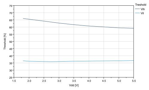
Figure 33-21. I/O Pin Input Threshold Voltage vs.  $V_{DD}$  ( $V_{IH}$ )
