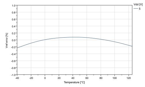
Figure 33-37. Internal 4.3V Reference vs. Temperature
