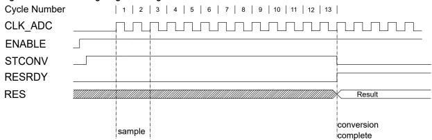
Both sampling time and sampling length can be adjusted using the Sample Delay bit field in Control D (ADCn.CTRLD) and sampling Sample Length bit field in the Sample Control register (ADCn.SAMPCTRL). Both of these control the ADC sampling time in a number of CLK\_ADC cycles. This allows sampling high-impedance sources without relaxing conversion speed. See the register description for further information. Total sampling time is given by:
