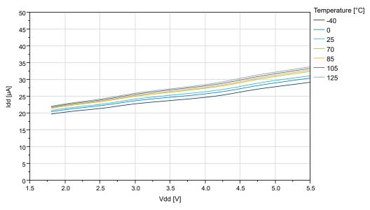
Figure 33-39. BOD Current vs.  $V_{DD}$  (Sampled BOD at 125 Hz)
