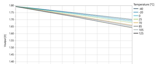
Figure 33-27. I/O Pin Output Voltage vs. Source Current ( $V_{DD} = 1.8V$ )
