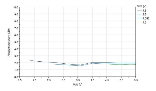
Figure 33-55. Absolute Accuracy vs.  $V_{REF}$  ( $V_{DD}$  = 5.0V,  $f_{ADC}$  = 115 ksps, REFSEL = External Reference)
