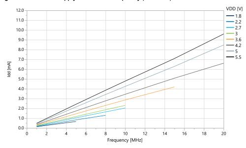
Figure 33-2. Active Supply Current vs. Frequency [0.1, 1.0] MHz at T = 25 °C
