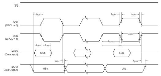
Figure 32-7. SPI - Timing Requirements in Slave Mode
