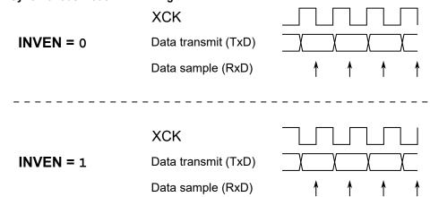
The I/O pin can be inverted by writing a '1' to the Inverted I/O Enable (INVEN) bit in the Pin n Control register of the port peripheral (PORTx.PINnCTRL). Using the inverted I/O setting for the corresponding XCK port pin, the XCK clock edges used for sampling RxD and transmitting on TxD can be selected. If the inverted I/O is disabled (INVEN = 0), the rising XCK clock edge represents the start of a new data bit, and the received data will be sampled at the falling
