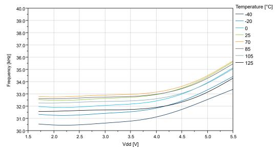
Figure 33-73. OSCULP32K Internal Oscillator: Frequency vs.  $V_{DD}$
