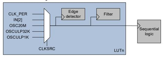
When the Clock Source (CLKSRC) bit is written to 0x1, IN[2] is used to clock the corresponding filter and edge detector (CLK\_LUTn). The sequencer is clocked by the CLK\_LUTn of the even LUT in the pair. When CLKSRC is written to 0x1, IN[2] is treated as OFF (low) in the TRUTH table.
