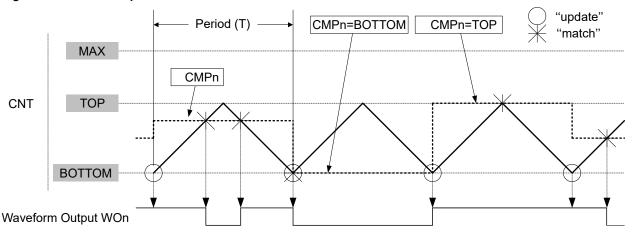
Using dual-slope PWM results in half the maximum operation frequency compared to single-slope PWM operation, due to twice the number of timer increments per period.
