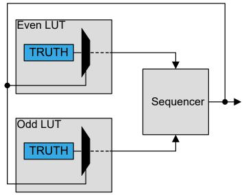
When selected (INSELy=FEEDBACK in LUTnCTRLx), the sequencer (SEQ) output is used as input for the corresponding LUTs.
