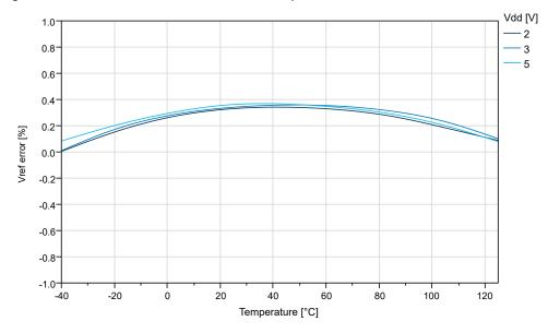
Figure 33-35. Internal 1.1V Reference vs. Temperature
