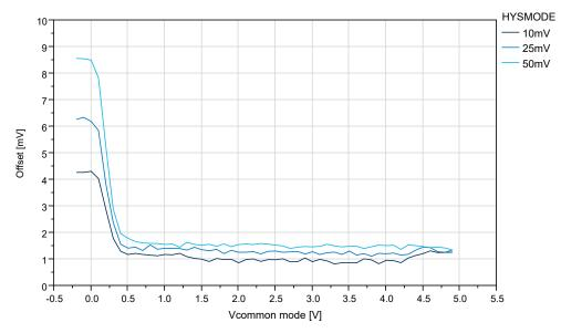
Figure 33-67. Offset vs.  $V_{CM}$  - 10 mV to 50 mV ( $V_{DD}$  = 5V, T = 25°C)
