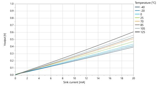
Figure 33-26. I/O Pin Output Voltage vs. Sink Current (T = 25°C)
