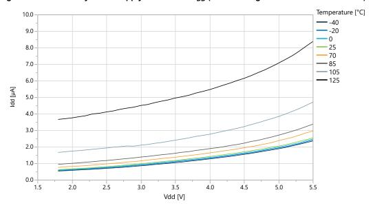
Figure 33-16. Standby Mode Supply Current vs. V<sub>DD</sub> (Sampled BOD running at 125 Hz)
