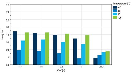
Figure 33-49. Gain Error vs.  $V_{REF}$  ( $V_{DD}$  = 5.0V,  $f_{ADC}$  = 115 ksps), REFSEL = Internal Reference
