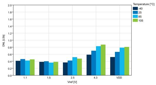
Figure 33-47. DNL vs.  $V_{REF}$  ( $V_{DD}$  = 5.0V,  $f_{ADC}$  = 115 ksps), REFSEL = Internal Reference
