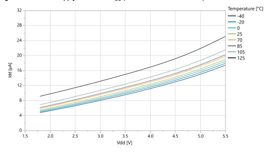
Figure 33-7. Active Supply Current vs. V<sub>DD</sub> (f = 32.768 kHz OSCULP32K)
