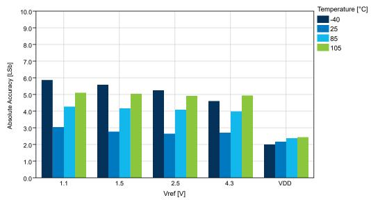
Figure 33-45. Absolute Accuracy vs.  $V_{REF}$  ( $V_{DD}$  = 5.0V,  $f_{ADC}$  = 115 ksps), REFSEL = Internal Reference
