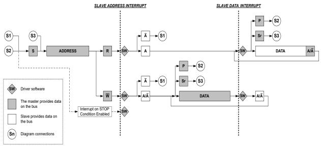
The number of interrupts generated is kept to a minimum by automatic handling of most conditions. The Quick command can be enabled to auto-trigger operations and reduce software complexity.
