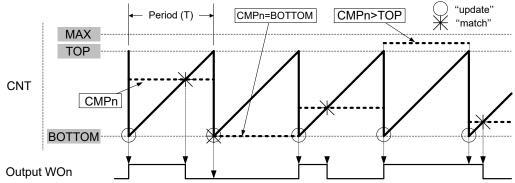
The TCAn.PER register defines the PWM resolution. The minimum resolution is 2 bits (TCA.PER = 0x0002), and the maximum resolution is 16 bits (TCA.PER = MAX-1).
