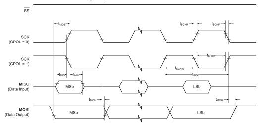
Table 32-18. USART in SPI Master Mode - Timing Characteristics<sup>(1)</sup>
