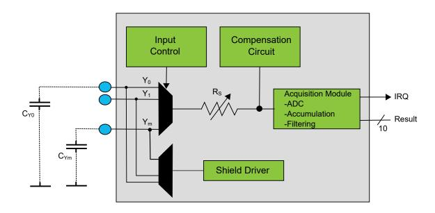
**Note:** The internal series resistor,  $R_S$ , has limited effect in Self-Capacitance mode. It is always recommended to add an external series resistor.
