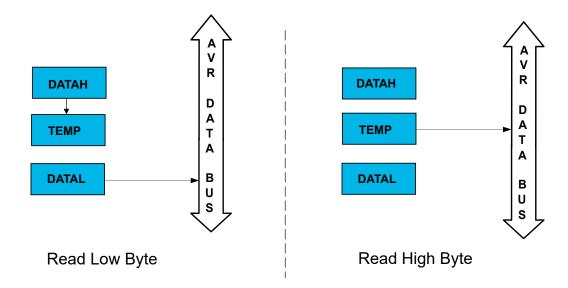
For a 16-bit read operation, the low byte register (e.g., DATAL) of the 16-bit register must be read before the high byte register (e.g., DATAH). When the low byte register is read, the high byte register of the 16-bit register is copied into the temporary (TEMP) register in the same clock cycle, as shown on the left side of Figure 7-3. Reading the high byte register will result in a read from TEMP instead of the high byte register, as shown on the right side of Figure 7-3.
