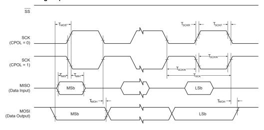
Table 37-19. SPI - Timing Characteristics in Master Mode
