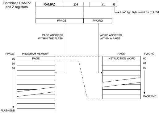
The Flash is word-accessed and organized in pages, so the Address Pointer can be treated as having two sections. This is shown in Figure 10-3. The word address in the page (FWORD) is held by the Least Significant bits in the Address Pointer, while the most significant bits in the Address Pointer hold the Flash page address (FPAGE). Together, FWORD and FPAGE hold an absolute address to a word in the Flash.
