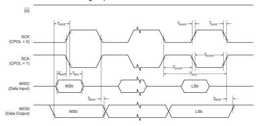
Table 37-18. USART in SPI Master Mode - Timing Characteristics
