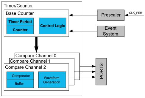
Figure 21-1. 16-bit Timer/Counter and Closely Related Peripherals
