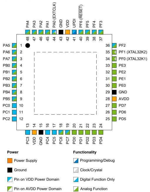
**Note:** For the AVR® DA Family, the VDD and AVDD are internally connected (no separate power domains).
