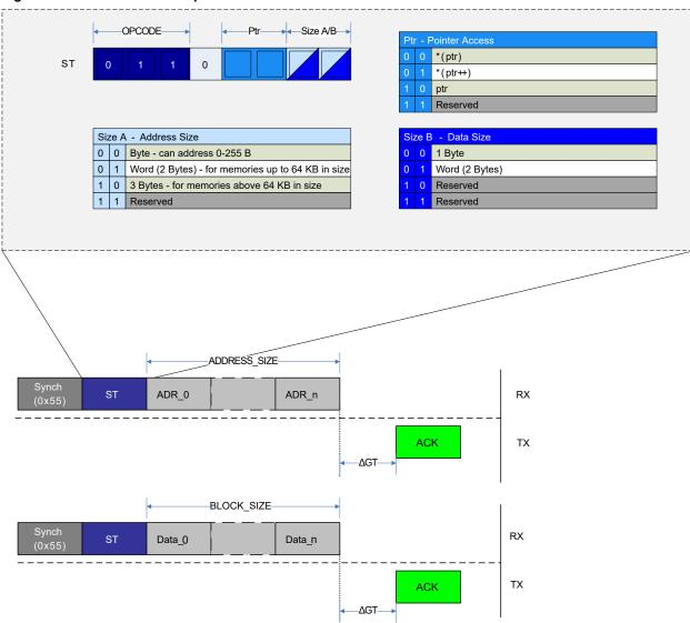
The figure above gives an example of an ST instruction to the UPDI Pointer register and the storage of regular data. A SYNCH character is sent before each instruction. In both cases, an Acknowledge (ACK) is sent back by the UPDI if the ST instruction was successful.
