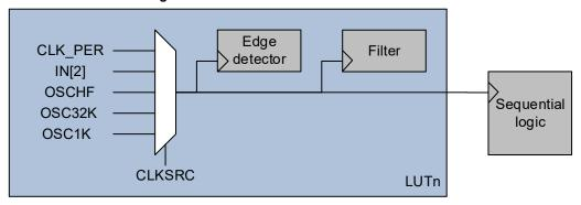
When the Clock Source (CLKSRC) bit is written to 0x1, LUTn-TRUTHSEL[2] is used to clock the corresponding filter and edge detector (CLK\_LUTn). The sequencer is clocked by the CLK\_LUTn of the even LUT in the pair. When CLKSRC is written to 0x1, LUTn-TRUTHSEL[2] is treated as OFF (low) in the TRUTH table.
