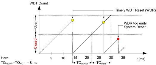
The Window mode is enabled by writing a non-zero value to the Window (WINDOW) bit field in the Control A (WDT.CTRLA) register. The Window mode is disabled by writing the WINDOW bit field to '0x0'.
