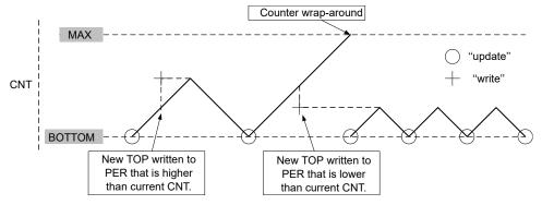
**With Buffering:** When double-buffering is used, the buffer can be written at any time and still maintain correct operation. The TCAn.PER is always updated on the UPDATE condition, as shown for dual-slope operation in the figure below. This prevents wrap-around and the generation of odd waveforms.
