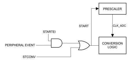
In Free-Running mode, the first conversion is started by writing a '1' to the STCONV bit in the ADCn.COMMAND register. A new conversion cycle is started immediately after the previous conversion cycle has completed. A completed conversion will set the RESRDY flag in the ADCn.INTFLAGS register.
