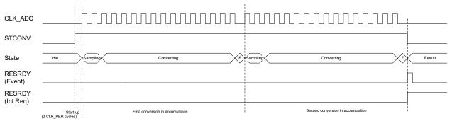
The number of samples to accumulate is configured with the Sample Number (SAMPNUM) bit field in the Control B (ADCn.CTRLB) register. The STCONV bit is set for the entire conversion. The total conversion time for n samples is given by:
