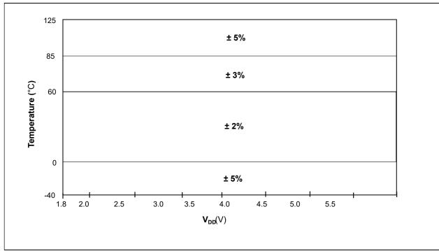
Table 37-11. 32.768 kHz External Crystal Oscillator (XOSC32K) Characteristics
