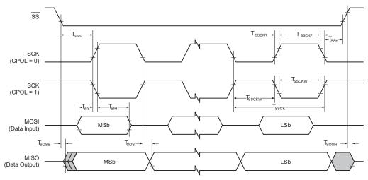
Table 37-20. SPI - Timing Characteristics in Slave Mode
