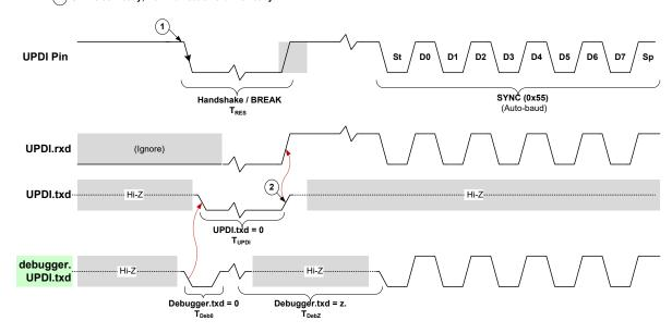
To avoid the UPDI from staying enabled if an accidental trigger of the edge detector happens, the UPDI will automatically disable itself and lower its clock request. See the *Disable During Start-up* section for more details.
