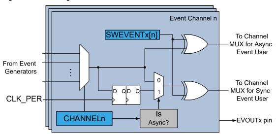
The block diagram shows the operation of an event channel. A multiplexer controlled by Channel n Generator Selection (EVSYS.CHANNELn) register at the input selects which of the event sources to route onto the event channel. Each event channel has two subchannels: one asynchronous and one synchronous. A synchronous user will listen to the synchronous subchannel, and an asynchronous user will listen to the asynchronous subchannel.
