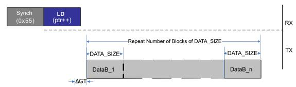
For LD, data will come out continuously after the LD instruction. Note the guard time on the first data block.
