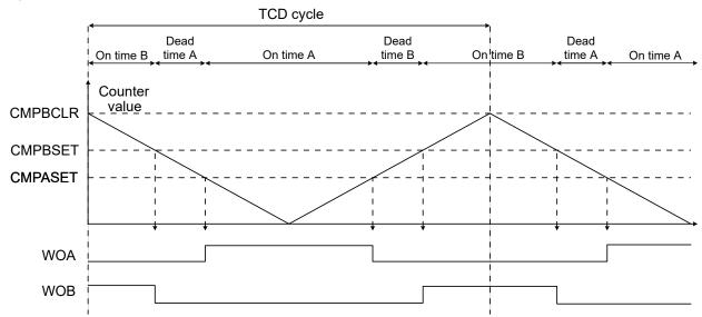
When starting the TCD in Dual Slope mode, the TCD counter starts at the CMPBCLR value and counts down. In the first cycle, the WOB will not be set until the TCD counter matches the CMPBSET value when counting up.
