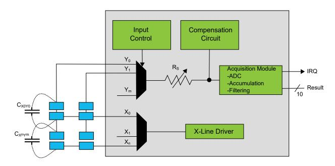
Figure 33-2. PTC Block Diagram in Self-Capacitance Mode
