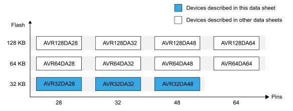
Devices with different Flash memory sizes typically also have different SRAM.
