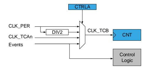
The Clock Select (CLKSEL) bit field in the Control A (TCBn.CTRLA) register selects one of the prescaler outputs directly, or an event channel as the clock (CLK\_TCB) input.
