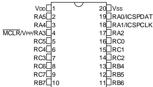
**Figure 3.****20-Pin VQFN**
