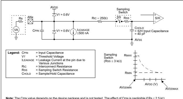
Note: The CPIN value depends on the device package and is not tested. The effect of CPIN is negligible if Rs  $\leq$  2.5 k $\Omega$ .
