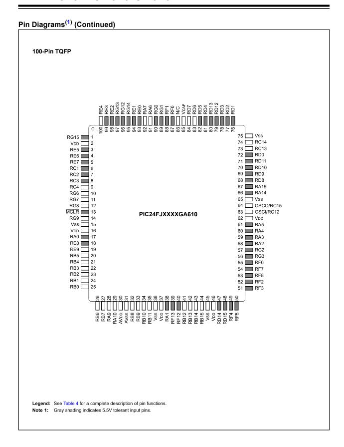
TABLE 4: COMPLETE PIN FUNCTION DESCRIPTIONS (PIC24FJXXXGA610 TQFP)
