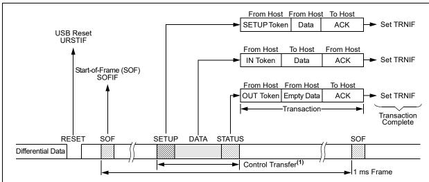
**Note 1:** The control transfer shown here is only an example showing events that can occur for every transaction. Typical control transfers will spread across multiple frames.
