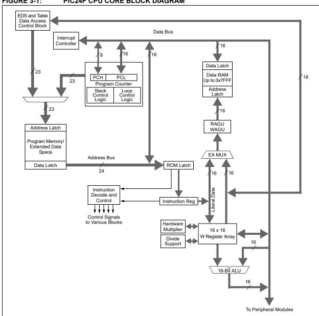
FIGURE 3-1: PIC24F CPU CORE BLOCK DIAGRAM
