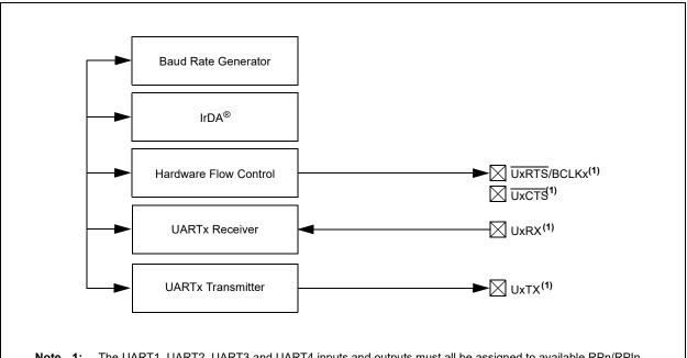
Note 1: The UART1, UART2, UART3 and UART4 inputs and outputs must all be assigned to available RPn/RPIn pins before use. See Section 11.4 "Peripheral Pin Select (PPS)" for more information.
