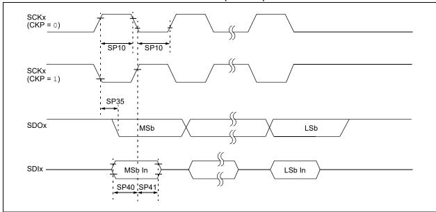
FIGURE 33-11: SPIX MODULE MASTER MODE (CKE = 1) TIMING CHARACTERISTICS
