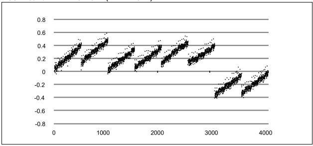
FIGURE 33-21: DNL vs. CODE (12-BIT MODE)<sup>(1)</sup>
