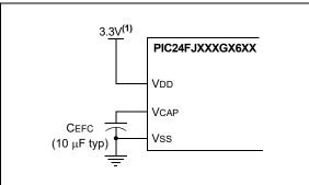
Note 1: This is a typical operating voltage. Refer to Section 33.0 "Electrical Characteristics" for the full operating ranges of VDD.
