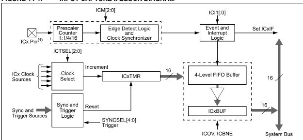
Note 1: The ICx input must be assigned to an available RPn/RPIn pin before use. See Section 11.4 "Peripheral Pin Select (PPS)" for more information.
