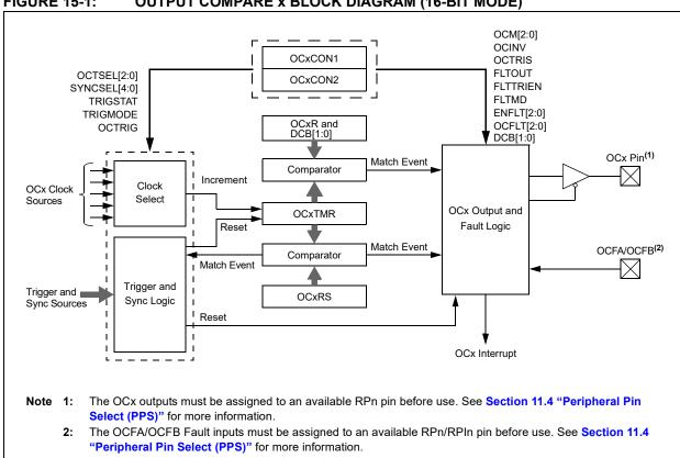
**FIGURE 15-1:** OUTPUT COMPARE x BLOCK DIAGRAM (16-BIT MODE)
