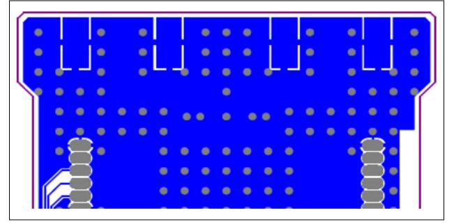
path is not used for this module. The host PCB can follow these trace designs to maintain compliance under the modular grant (FCC) and certificate (IC). Gerber files are available on the RN2903 product web page at www.microchip.com/rn2903.
