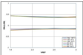
**FIGURE 36-63:** ADC 10-Bit Mode, Single-Ended DNL, VDD = 3.0V, TAD = 4 uS (All devices)
