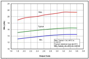
FIGURE 36-75: DAC INL Error, VDD = 3.0V (PIC16LF18326/46 only)
