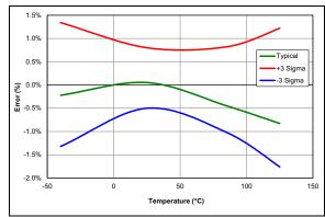
FIGURE 36-32: HFINTOSC Frequency Error VDD = 3V (All devices)
