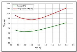
FIGURE 36-116: Wake From Sleep, VREGPM = 1, HFINTOSC = 16 MHz (PIC16F18326/46 only)
