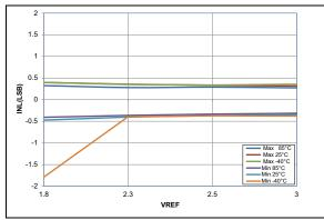
FIGURE 36-60: ADC 10-Bit Mode, Single-Ended INL, VDD = 3.0V, TAD = 1 uS (All devices)
