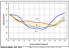
**FIGURE 36-83:** Comparator Hysteresis, Normal Power Mode (CxSP = 1), VDD = 5.5V, Typical Measured Values
