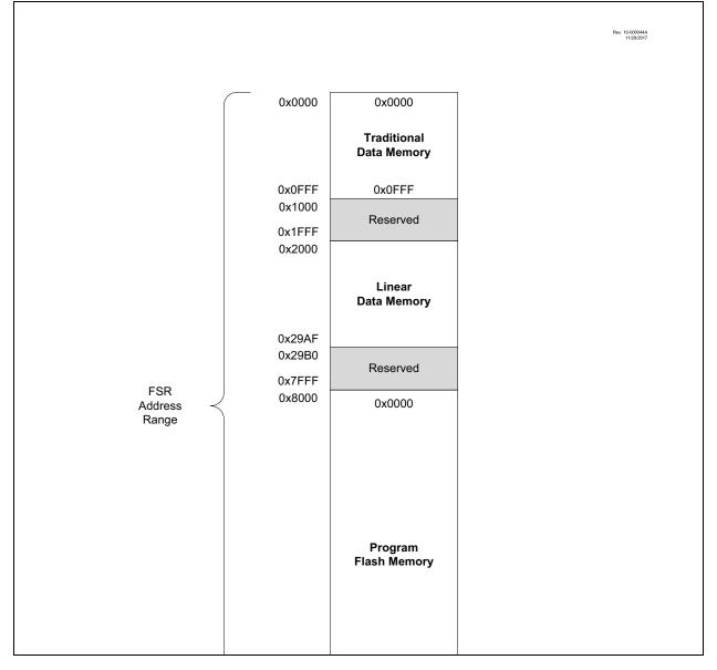
The traditional data memory is a region from FSR address 0x000 to FSR address 0xFFF. The addresses correspond to the absolute addresses of all SFR, GPR and common registers.
