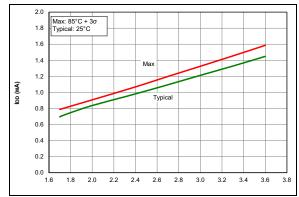
FIGURE 36-22: IDD, HFINTOSC Mode, Fosc = 16 MHz (PIC16LF18326/46 only)
