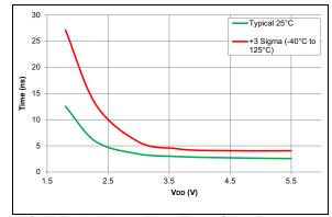
FIGURE 36-106: Rise Time, Slew Rate Control Disabled
