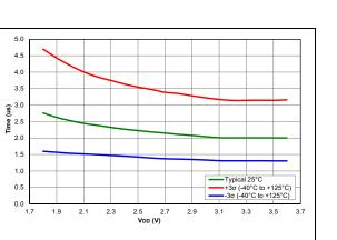
FIGURE 36-69: ADC RC Oscillator Period (PIC16LF18326/46 only)
