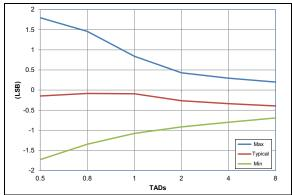
**FIGURE 36-68:** ADC 10-Bit Mode, Single-Ended Offset Error, VDD = 3.0V, VREF = 3.0V, -40°C to 85°C(All devices)
