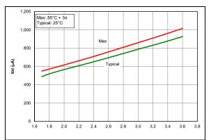
FIGURE 36-26: IDD, HFINTOSC Doze Mode, Fosc = 16 MHz (PIC16LF18326/46 only)
