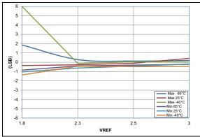
FIGURE 36-61: ADC 10-Bit Mode, Single-Ended Gain Error, VDD = 3.0V, TAD = 1 uS (All devices)
