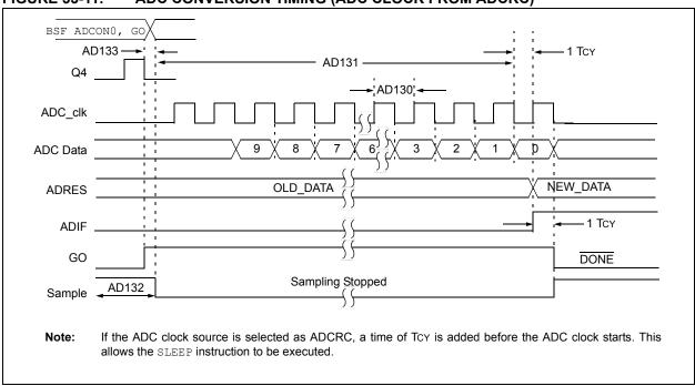
FIGURE 35-11: ADC CONVERSION TIMING (ADC CLOCK FROM ADCRC)
