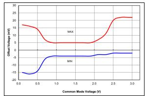
**FIGURE 36-82:** Comparator Offset, Normal Power Mode (CxSP = 1), VDD = 3.0V, Typical Measured Values from -40°C to 125°C
