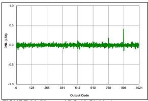
FIGURE 36-53: ADC 10-Bit Mode, Single-Ended DNL, VDD = 3.0V, VREF = 3.0V, TAD = 8 uS, 25C (All devices)
