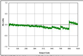
FIGURE 36-56: ADC 10-Bit Mode, Single-Ended INL, VDD = 3.0V, VREF = 3.0V, TAD = 8 uS, 25C (All devices)
