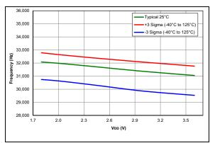
FIGURE 36-28: LFINTOSC Frequency (PIC16LF18326/46 only)
