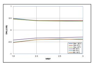
**FIGURE 36-59:** ADC 10-Bit Mode, Single-Ended DNL, VDD = 3.0V, TAD = 1 uS (All devices)
