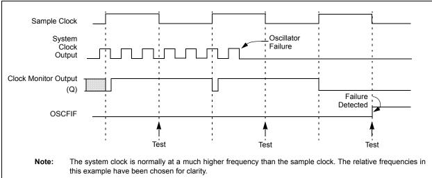
FIGURE 7-10: FSCM TIMING DIAGRAM
