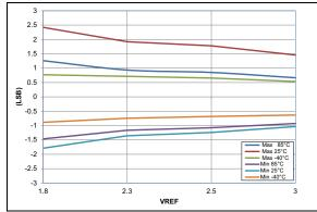
**FIGURE 36-62:** ADC 10-Bit Mode, Single-Ended Offset Error, VDD = 3.0V, TAD = 1 uS (All devices)
