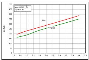
FIGURE 36-16: IDD, XT Oscillator 4 MHz (PIC16LF18326/46 only)
