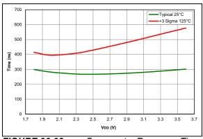
FIGURE 36-92: Comparator Response Time Rising Edge
