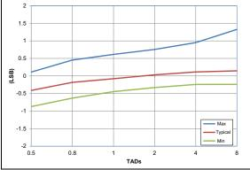
**FIGURE 36-67:** ADC 10-Bit Mode, Single-Ended Gain Error, VDD = 3.0V, VREF = 3.0V, -40°C to 85°C(All devices)
