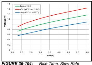
FIGURE 36-104: Rise Time, Slew Rate Control Enabled
