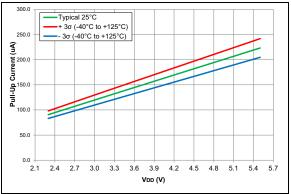
FIGURE 36-33: Weak Pull-Up Current (PIC16F18326/46 only)
