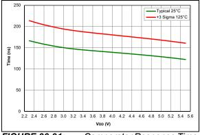
FIGURE 36-91: Comparator Response Time Falling Edge
