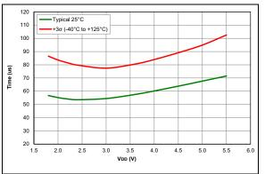
FIGURE 36-114: Wake From Sleep, VREGPM = 1, HFINTOSC = 4 MHz (PIC16F18326/46 only)
