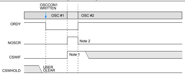
Note 1: CSWIF is asserted coincident with NOSCR; interrupt is serviced at OSC#2 speed.2: The assertion of NOSCR is hidden from the user because it appears only for the duration of the switch.
