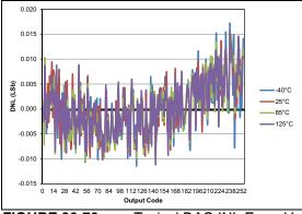
FIGURE 36-73: Typical DAC INL Error, VDD = 5.0V, VREF = External 5V (PIC16F18326/46 only)
