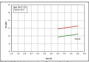
**FIGURE 36-8:** IPD, Brown-Out Reset (BOR), BORV = 1 (PIC16LF18326/46 only)
