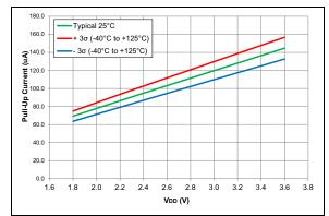
FIGURE 36-34: Weak Pull-Up Current (PIC16LF18326/46 only)
