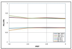
FIGURE 36-64: ADC 10-Bit Mode, Single-Ended INL, VDD = 3.0V, TAD = 4 uS (All devices)
