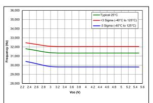
FIGURE 36-29: LFINTOSC Frequency (PIC16F18326/46 only)
