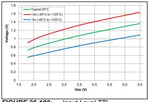
FIGURE 36-103: Input Level TTL
