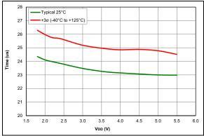
FIGURE 36-115: Wake From Sleep, VREGPM = 1, HFINTOSC = 16 MHz (PIC16F18326/46 only)
