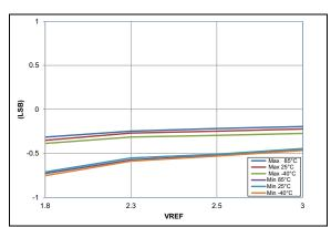
**FIGURE 36-66:** ADC 10-Bit Mode, Single-Ended Offset Error, VDD = 3.0V, TAD = 4 uS (All devices)
