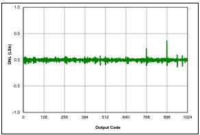
**FIGURE 36-52:** ADC 10-Bit Mode, Single-Ended DNL, VDD = 3.0V, VREF = 3.0V, TAD = 4 uS, 25C (All devices)
