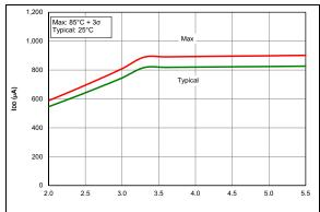
FIGURE 36-25: IDD, HFINTOSC Idle Mode, Fosc = 16 MHz (PIC16F18326/46 only)
