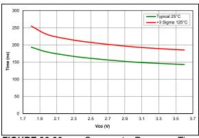
FIGURE 36-90: Comparator Response Time Falling Edge
