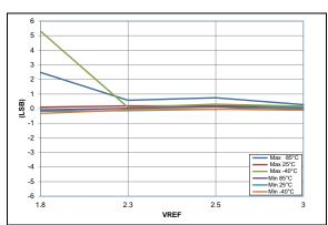
FIGURE 36-65: ADC 10-Bit Mode, Single-Ended Gain Error, VDD = 3.0V, TAD = 4 uS (All devices)
