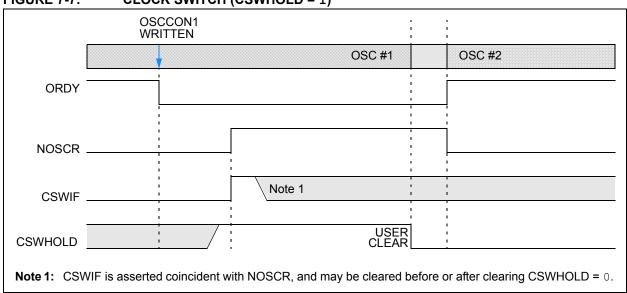
FIGURE 7-7: CLOCK SWITCH (CSWHOLD = 1)
