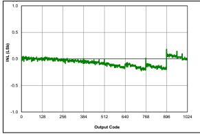
**FIGURE 36-55:** ADC 10-Bit Mode, Single-Ended INL, VDD = 3.0V, VREF = 3.0V, TAD = 4 uS, 25C (All devices)
