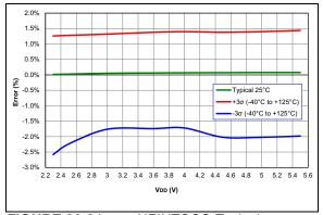
FIGURE 36-31: HFINTOSC Typical Frequency Error (PIC16F18326/46 only)
