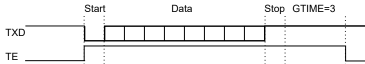
Figure 34-16. Example of TE Drive with Guard Time
