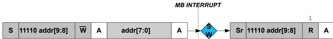
Figure 36-9. 10-bit Address Transmission for a Read Transaction
