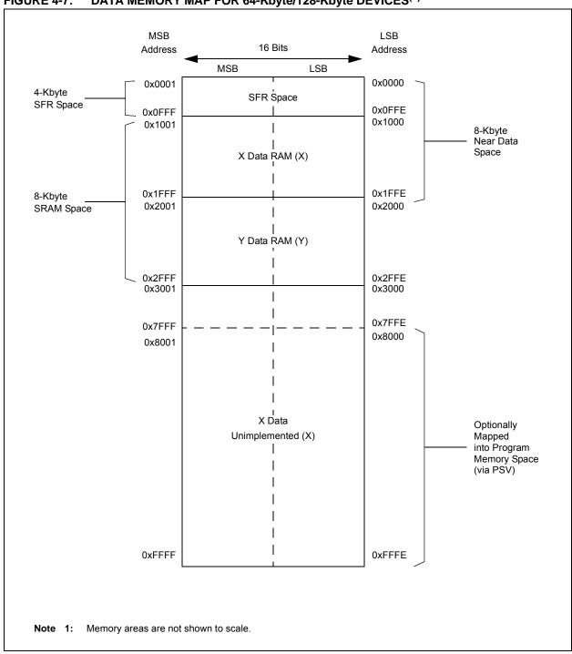
FIGURE 4-7: DATA MEMORY MAP FOR 64-Kbyte/128-Kbyte DEVICES<sup>(1)</sup>
