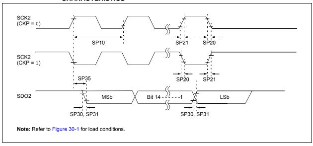
FIGURE 30-13: SPI2 MASTER MODE (HALF-DUPLEX, TRANSMIT ONLY, CKE = 1) TIMING CHARACTERISTICS
