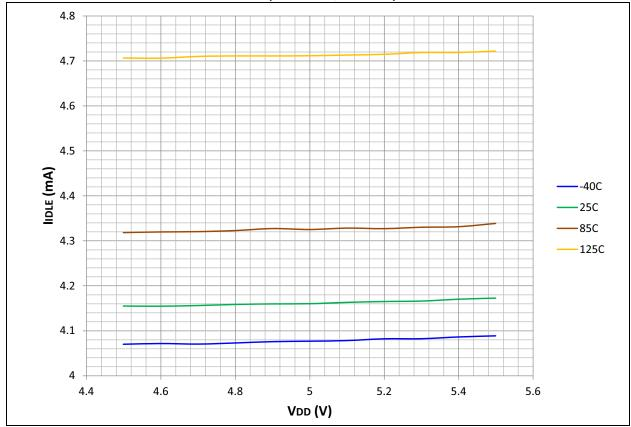
FIGURE 32-11: TYPICAL IIDLE vs. VDD (EC MODE, 60 MIPS)
