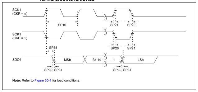
FIGURE 30-21: SPI1 MASTER MODE (HALF-DUPLEX, TRANSMIT ONLY, CKE = 1) TIMING CHARACTERISTICS
