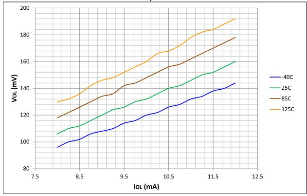
FIGURE 32-33: TYPICAL Vol 4x DRIVER PINS vs. Iol (GENERAL PURPOSE I/Os, **TEMPERATURES AS NOTED)**
