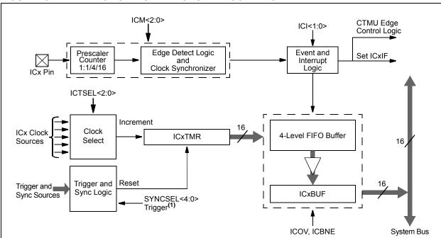
Note 1: The trigger/sync source is enabled by default and is set to Timer3 as a source. This timer must be enabled for proper ICx module operation or the trigger/sync source must be changed to another source option.
