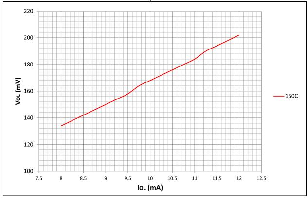
FIGURE 33-29: TYPICAL Vol 4x DRIVER PINS vs. Iol (GENERAL PURPOSE I/Os, **TEMPERATURES AS NOTED)**
