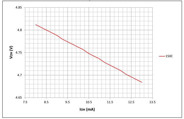
FIGURE 33-27: TYPICAL VOH 4x DRIVER PINS vs. IOH (GENERAL PURPOSE I/Os, TEMPERATURES AS NOTED)
