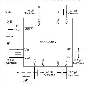
Note 1: As an option, instead of a hard-wired connection, an inductor (L1) can be substituted between VDD and AVDD to improve ADC noise rejection. The inductor impedance should be less than  $1\Omega$  and the inductor capacity greater than 10 mA.
