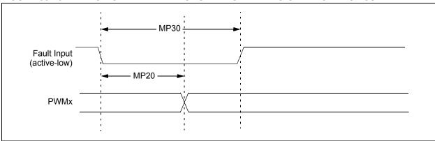
FIGURE 30-11: HIGH-SPEED PWMx MODULE TIMING CHARACTERISTICS
