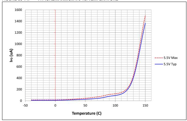
FIGURE 33-15: TYPICAL/MAXIMUM AIWDT vs. TEMPERATURE
