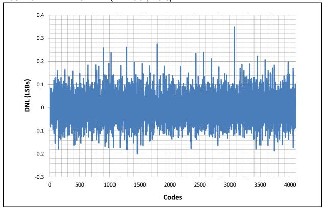
FIGURE 32-43: TYPICAL DNL (VDD = 5.5V, +85°C)
