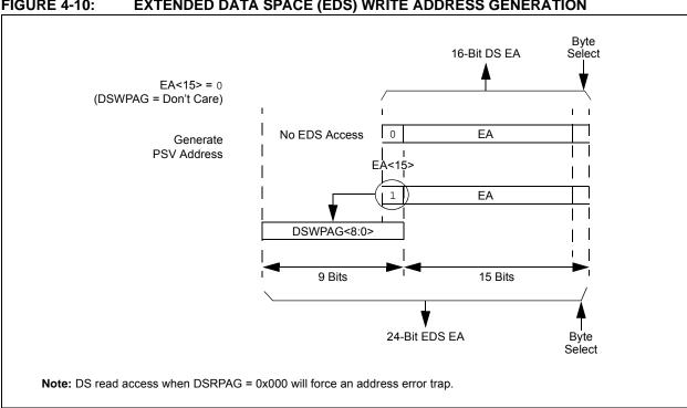
**FIGURE 4-10: EXTENDED DATA SPACE (EDS) WRITE ADDRESS GENERATION**
