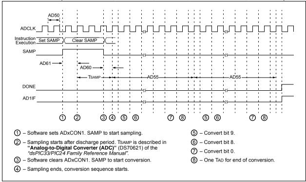
FIGURE 30-36: ADC CONVERSION (10-BIT MODE) TIMING CHARACTERISTICS (CHPS<1:0> = 01, SIMSAM = 0, ASAM = 1, SSRC<2:0> = 111, SSRCG = 0, SAMC<4:0> = 00010)
