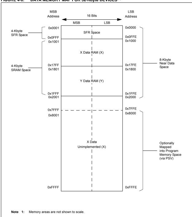
FIGURE 4-6: DATA MEMORY MAP FOR 32-Kbyte DEVICES<sup>(1)</sup>
