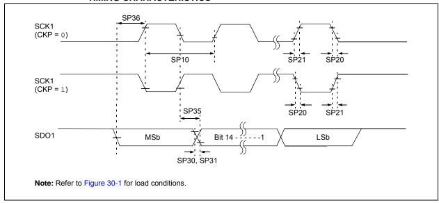
TABLE 30-39: SPI1 MASTER MODE (HALF-DUPLEX, TRANSMIT ONLY) TIMING REQUIREMENTS
