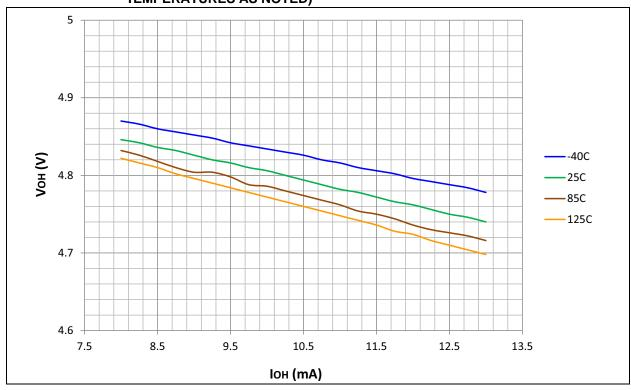
FIGURE 32-31: TYPICAL VOH 4x DRIVER PINS vs. IOH (GENERAL PURPOSE I/Os, TEMPERATURES AS NOTED)
