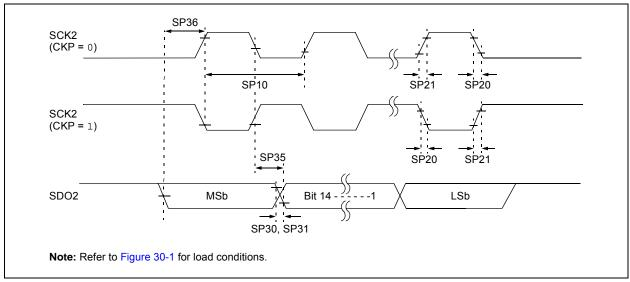
TABLE 30-31: SPI2 MASTER MODE (HALF-DUPLEX, TRANSMIT ONLY) TIMING REQUIREMENTS
