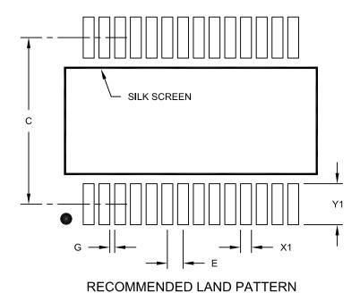
Units MILLIMETERS Dimension Limits MAX MIN MOM Contact Pitch 0.65 BSC Ε Contact Pad Spacing С 7.20 Contact Pad Width (X28) X1 0.45 Contact Pad Length (X28) Υ1 1.75 Distance Between Pads G 0.20
