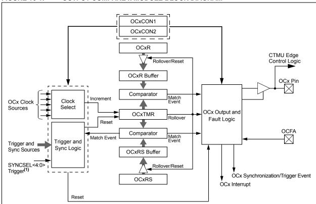
**Note 1:** The trigger/sync source is enabled by default and is set to Timer2 as a source. This timer must be enabled for proper OCx module operation or the trigger/sync source must be changed to another source option.
