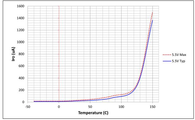
FIGURE 32-19: TYPICAL/MAXIMUM AIWDT vs. TEMPERATURE
