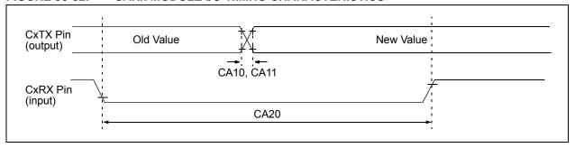
TABLE 30-48: CANX MODULE I/O TIMING REQUIREMENTS
