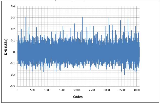
FIGURE 32-44: TYPICAL DNL (VDD = 5.5V, +125°C)
