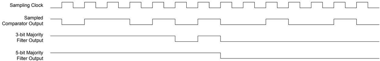
**Figure 29-7. Single-Shot Filtering**
