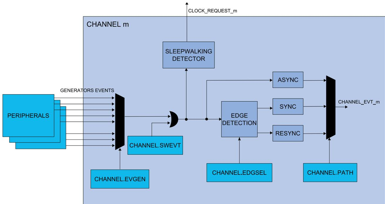
The path is selected by writing to the Path Selection bit group in the Channel register (CHANNEL.PATH).
