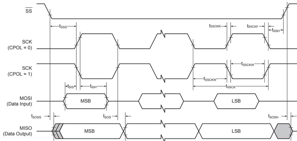
**Table 32-50. SPI timing characteristics and requirements<sup>(1)</sup>**
