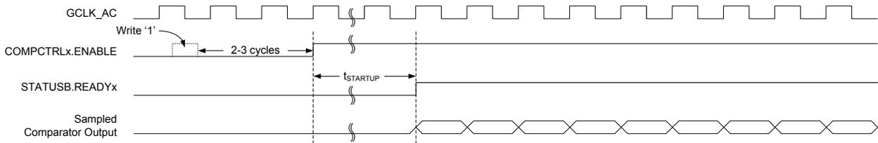
For low-power operation, comparisons can be performed during sleep modes without a clock. The comparator is enabled continuously, and changes of the comparator state are detected asynchronously. When a toggle occurs, the Power Manager will start CLK\_AC\_DIG to register the appropriate peripheral events and interrupts. The CLK\_AC\_DIG clock is then disabled again automatically, unless configured to wake up the system from sleep.
