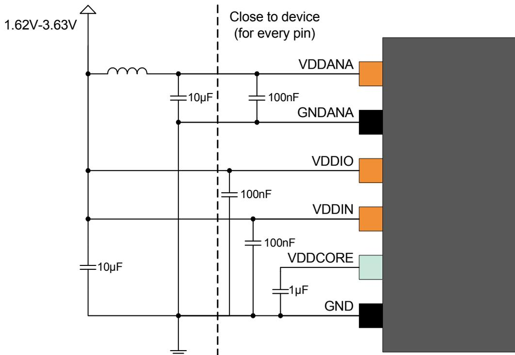
**Table 35-1. Power Supply Connections,  $V_{DDCORE}$  From Internal Regulator**
