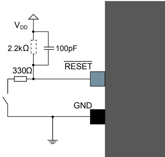
A pull-up resistor makes sure that the reset does not go low and unintentionally cause a device reset. An additional resistor has been added in series with the switch to safely discharge the filtering capacitor, i.e., preventing a current surge when shorting the filtering capacitor which again can cause a noise spike that can have a negative effect on the system.
