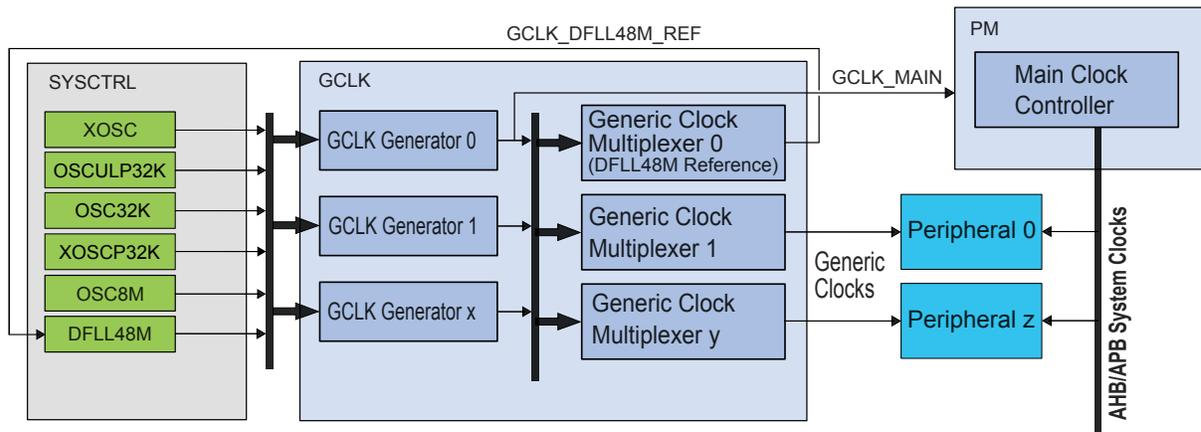
The clock system on the SAM D20 consists of:
