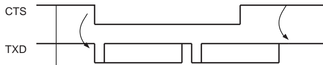
Figure 47-28: Transmitter Behavior when Operating with Hardware Handshaking
