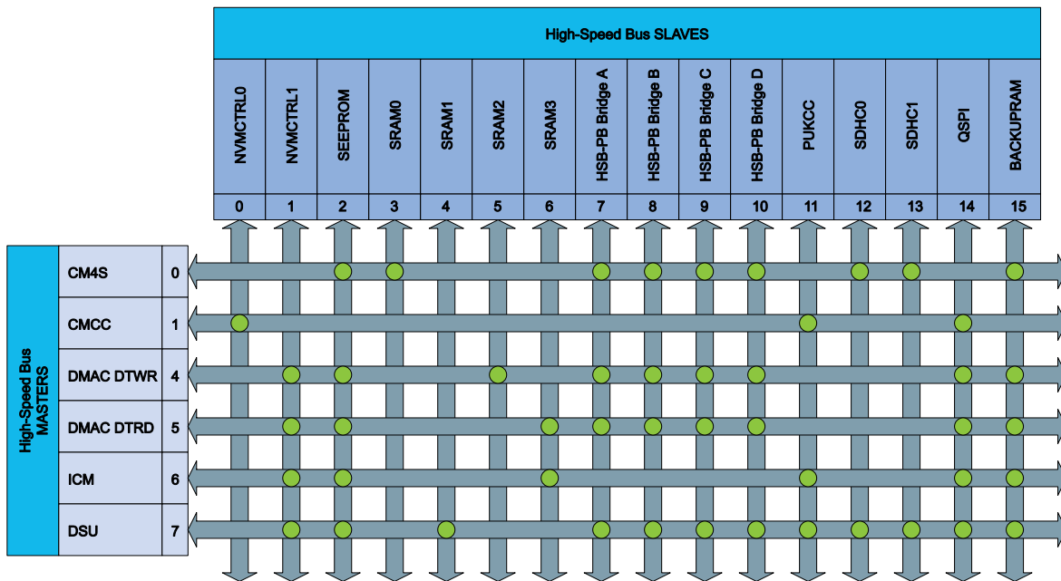
Figure 10-1. Master-Slave Relations High-Speed Bus Matrix
