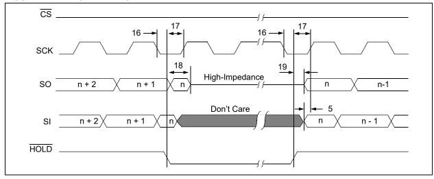
FIGURE 1-2: SERIAL INPUT TIMING
