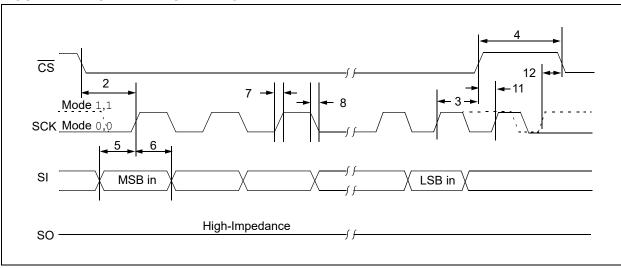
FIGURE 1-3: SERIAL OUTPUT TIMING
