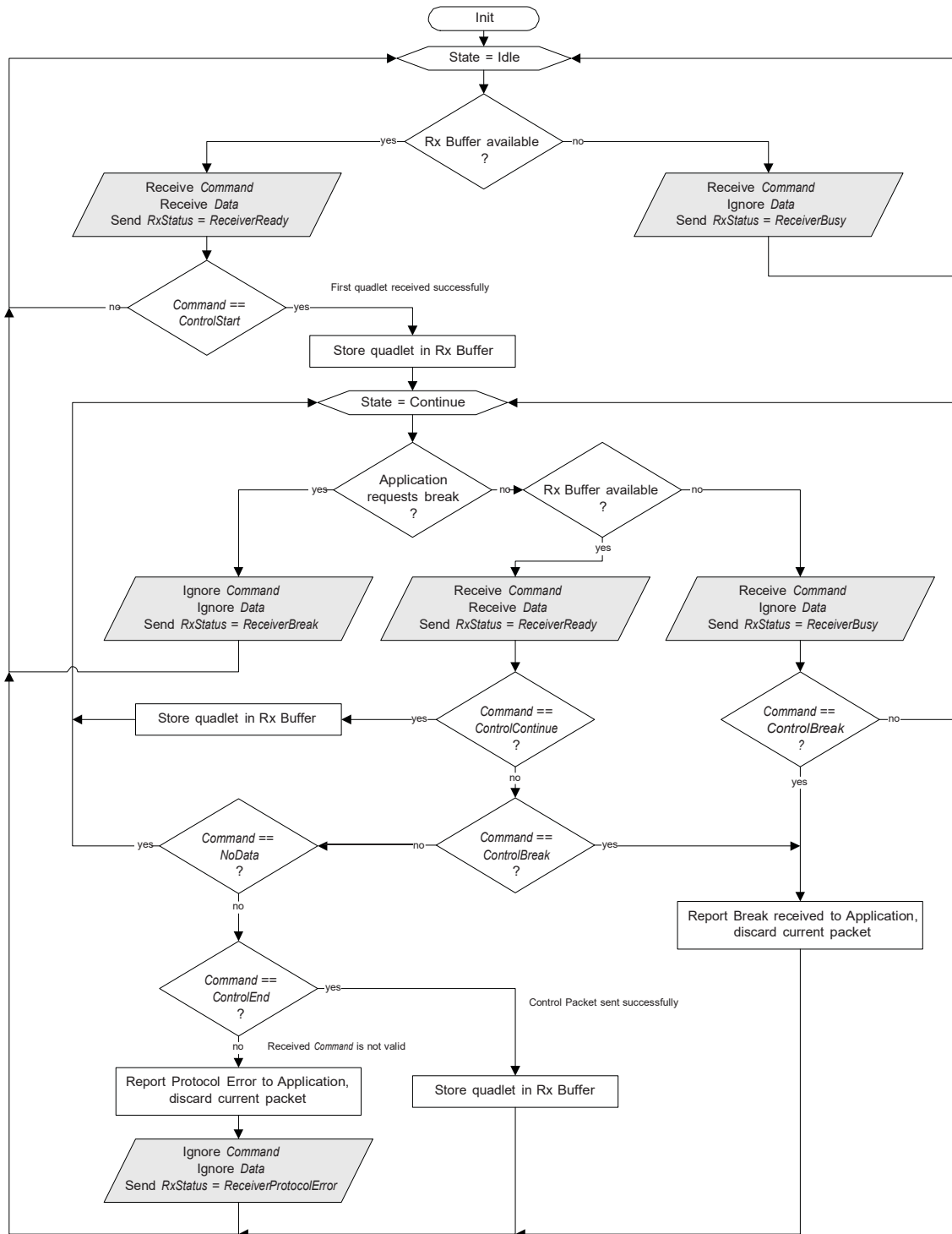
Figure 48-9. Control Packet Rx Device Protocol
