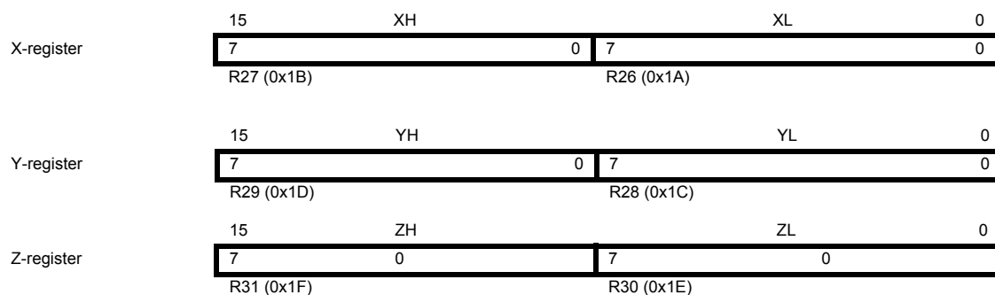
Figure 7-3. The X-, Y-, and Z-registers
