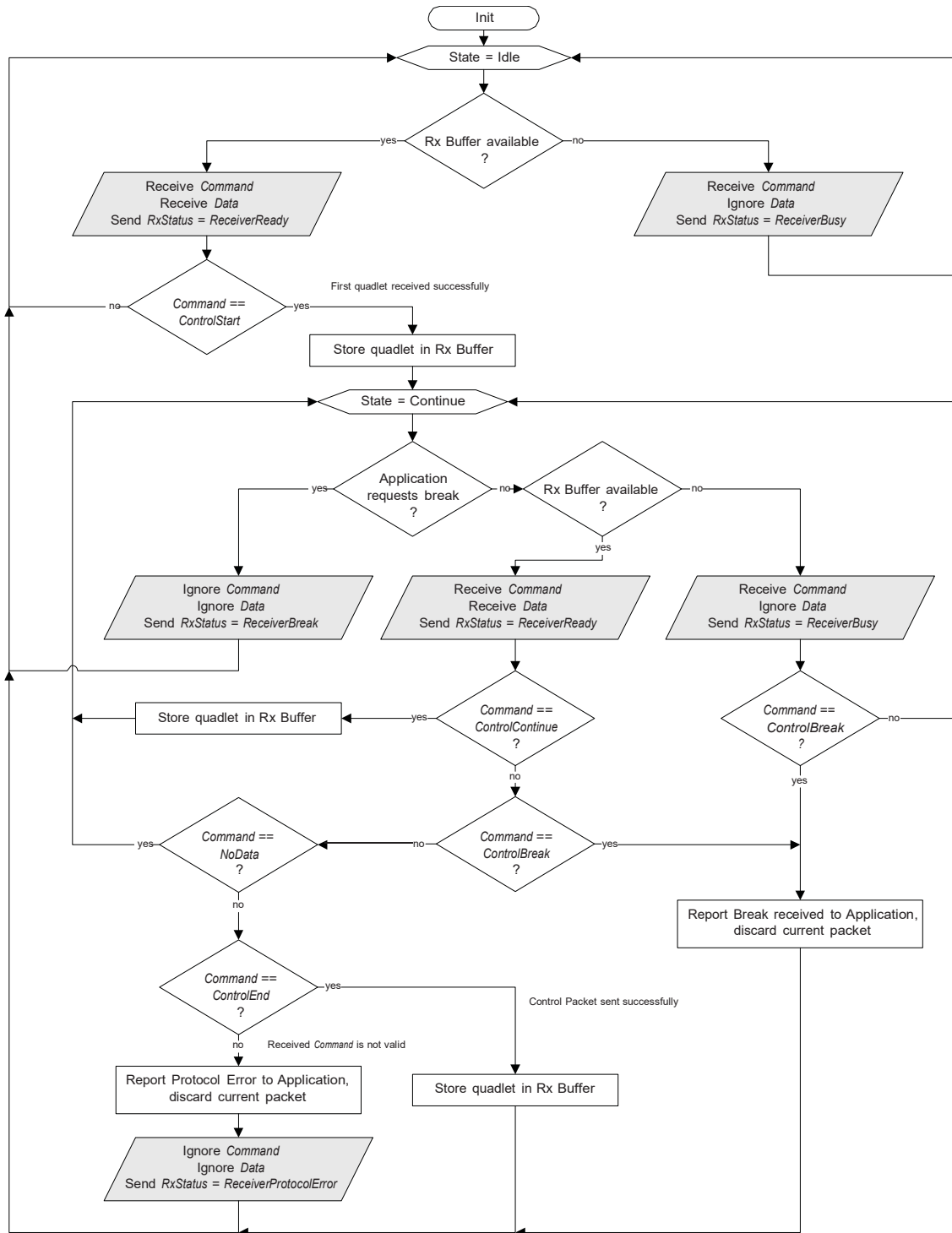
Figure 48-9. Control Packet Rx Device Protocol
