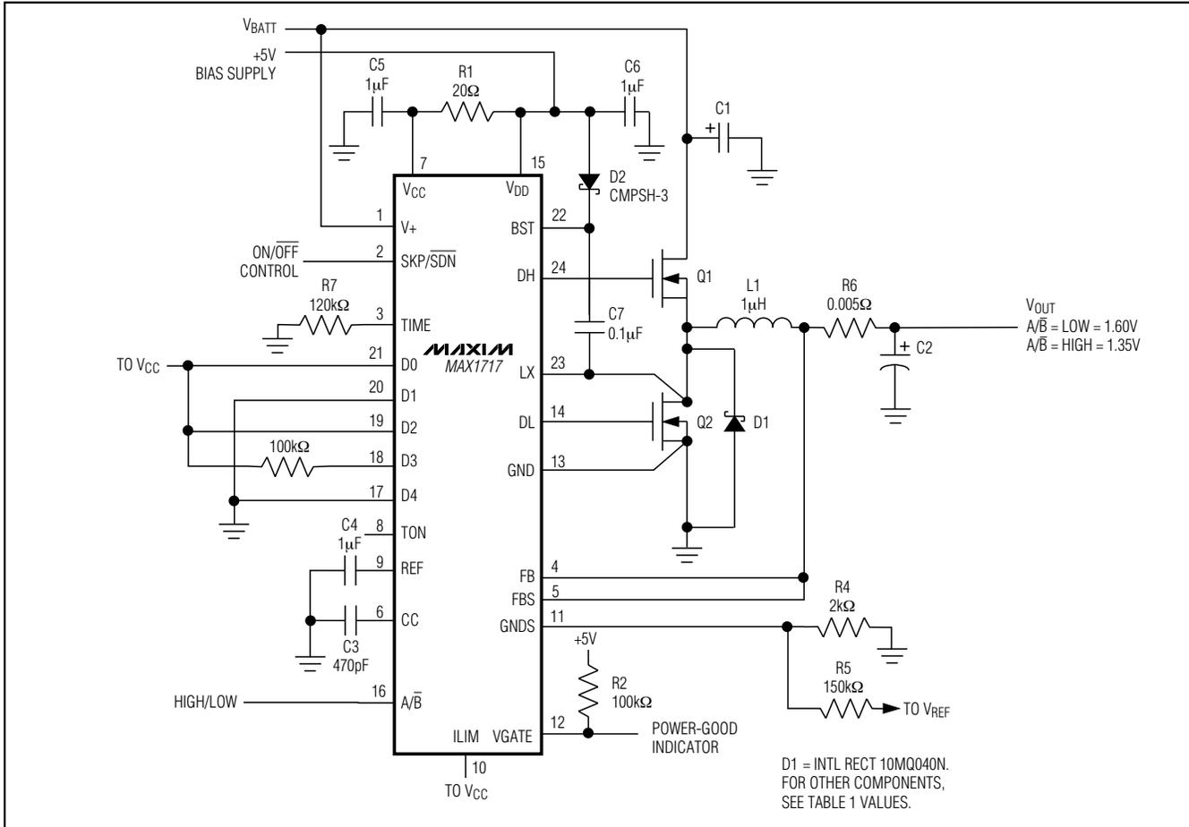
Figure 3. Voltage-Positioned Circuit
