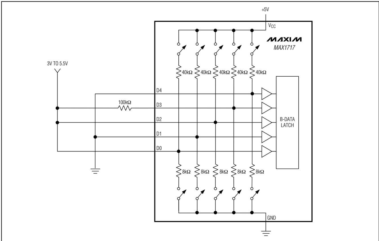
Figure 8. Internal Mux B-Mode Data Test and Latch
