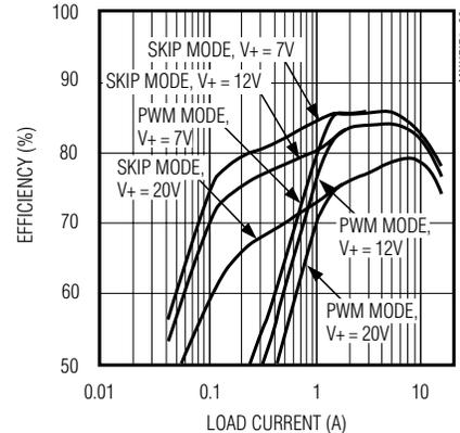
**EFFECTIVE EFFICIENCY vs. LOAD CURRENT
