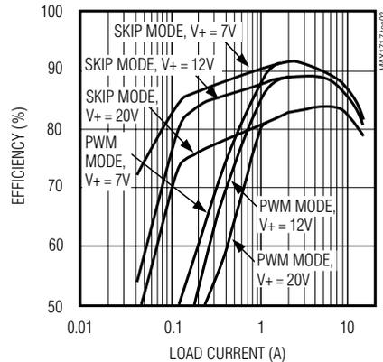
**EFFECTIVE EFFICIENCY vs. LOAD CURRENT
