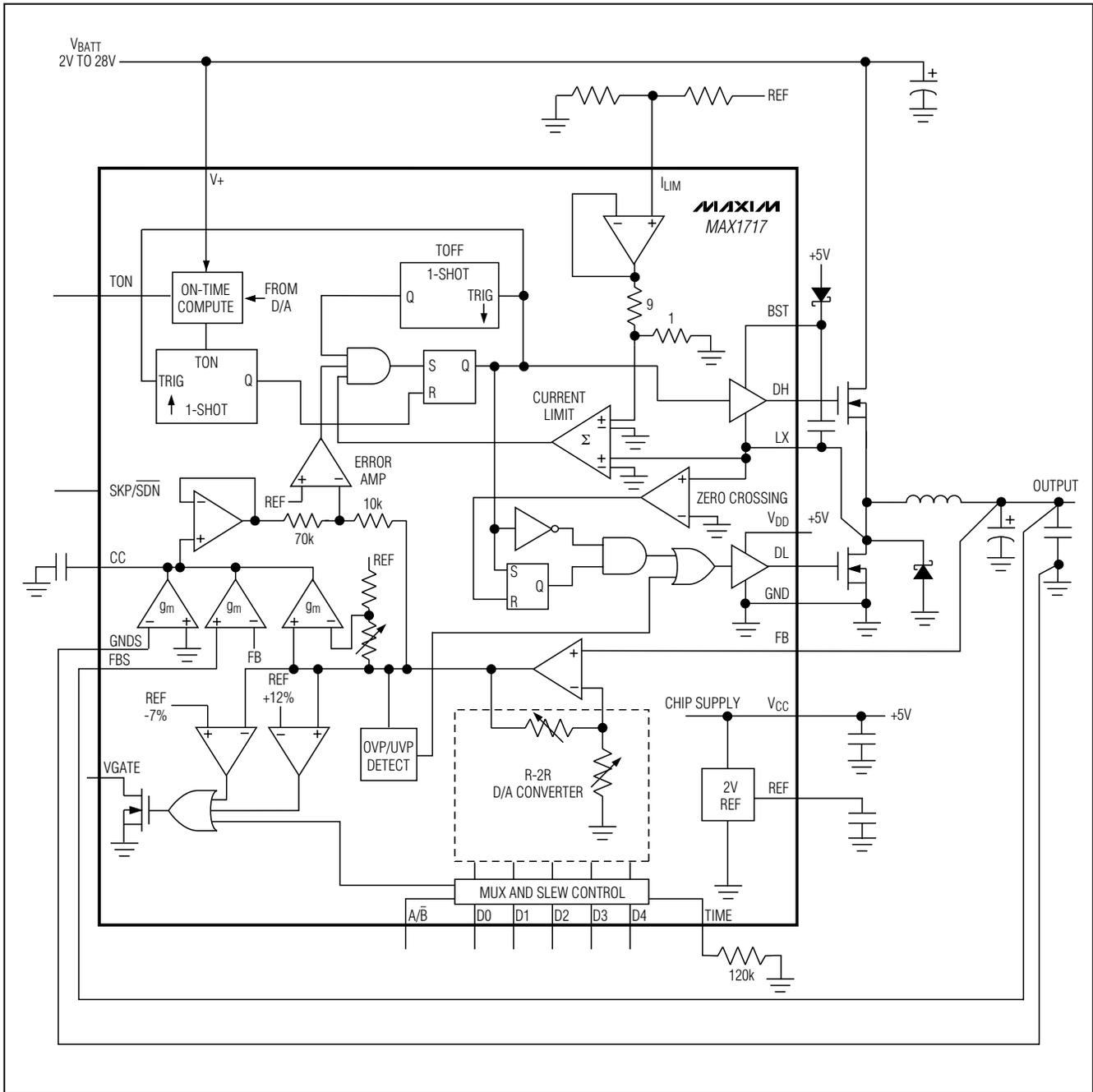
Figure 2. Functional Diagram
