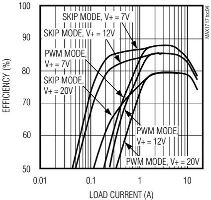
**EFFECTIVE EFFICIENCY vs. LOAD CURRENT
