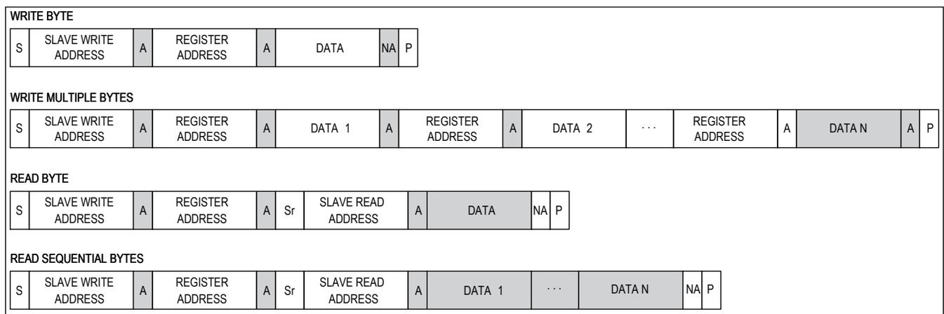
Figure 4. Data Format of I<sup>2</sup>C Interface
