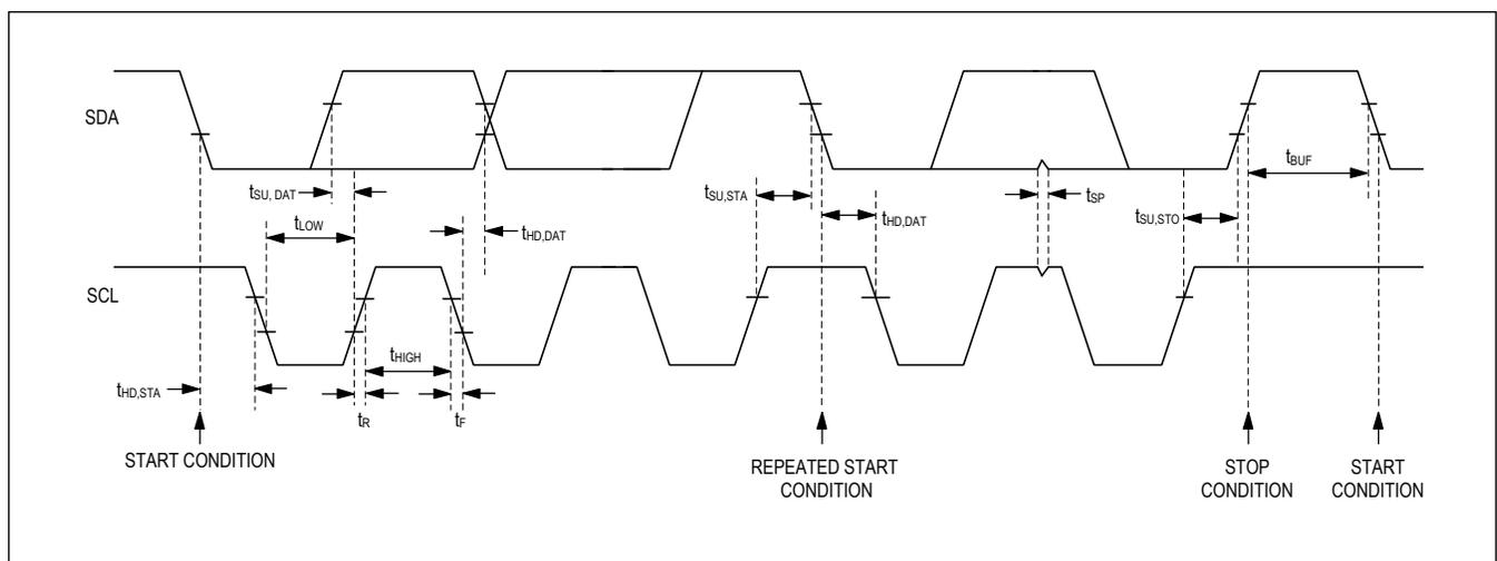
Figure 1. I<sup>2</sup>C Timing Diagram
