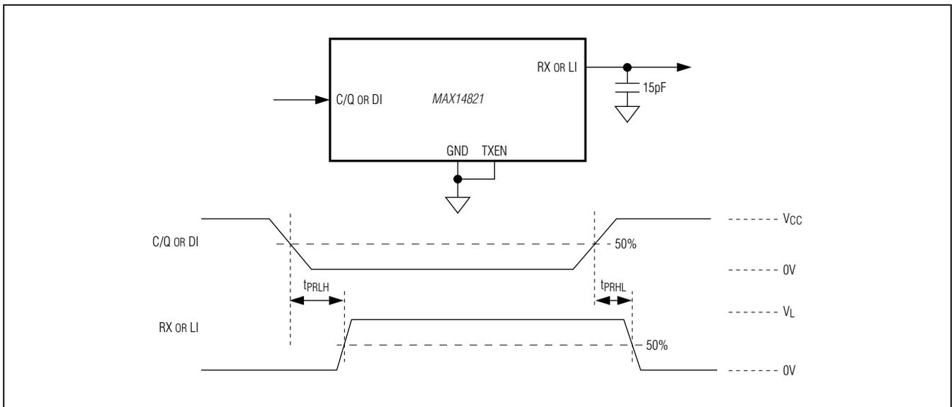
Figure 4. C/Q and DI Receiver Propagation Delays
