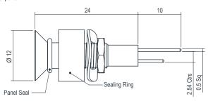
\* Min/max panel thickness is 3mm / 6.5mm
