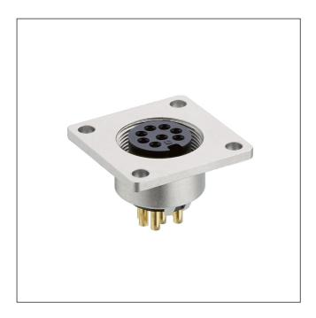
SWUM™ flange chassis socket acc. to IEC 61076-2-106 and AISG specification, IP68/67, with threaded joint and solder terminals, for front mounting
