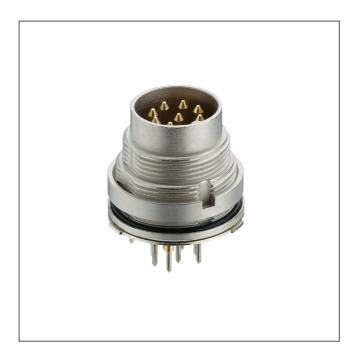
SWUM™ chassis plug acc. to IEC 61076-2-106 and AISG specification, IP68/67, with threaded joint and ground contact, for printed circuit boards, manual soldering, for back side mounting
