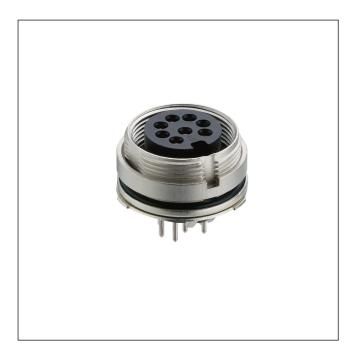
SWUM™ chassis socket acc. to IEC 61076-2-106 and AISG specification, IP68/67, with threaded joint and ground contact, for printed circuit boards, manual soldering, for back side mounting
