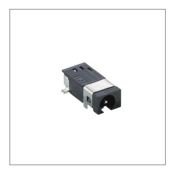
Power supply chassis socket acc. to JEITA RC-5320A JSAJ11, angular version, with break contact, for printed circuit boards, surface mount technology (SMT)
