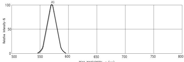
PEAK WAVELENGTH p (nm) Fig1.Spectral Emission
