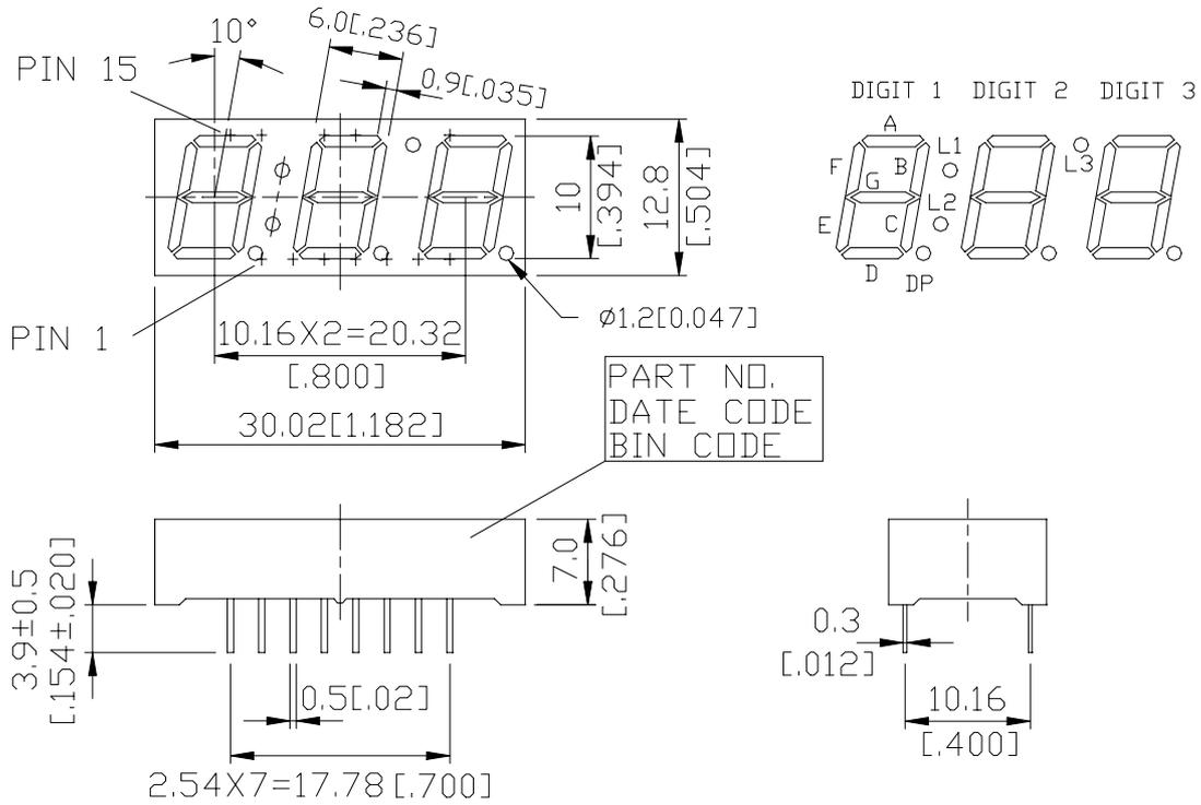
NOTES: All dimensions are in millimeters. Tolerances are ± 0.25 mm (0.01") unless otherwise noted.
