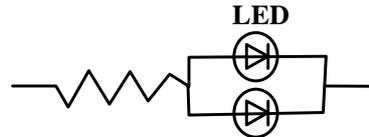
(B) The brightness of each LED might appear different due to the differences in the I-V characteristics of those LEDs.
