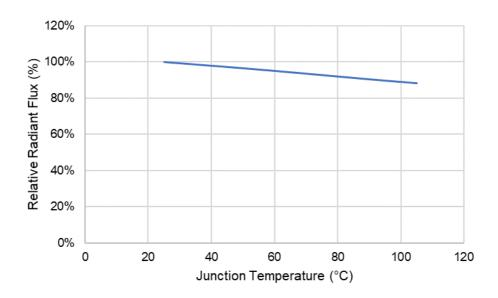
Fig.4 Relative Radiant Flux vs Junction Temperature
