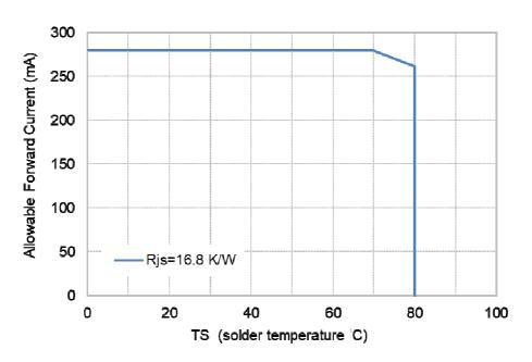
Fig 6. Forward Current Derating Curve
