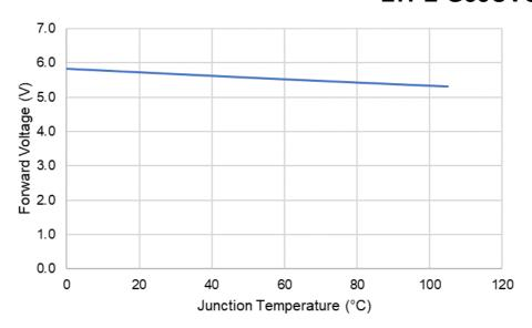
Fig.7 Forward Voltage vs Junction Temperature
