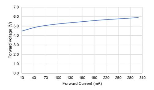
Fig 3. Forward Current vs. Forward Voltage
