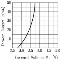
Forward Voltage V<sub>F</sub> (V) Fig.2 Forward Current vs. Forward Voltage
