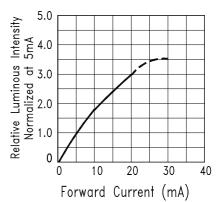
Fig.4 Relative Luminous Intensity vs. Forward Current
