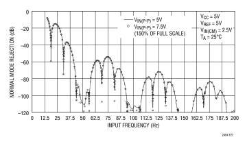
Figure 27. Measure Input Normal Mode Rejection vs Input Frequency With input Perturbation of 150% (50Hz Notch)
