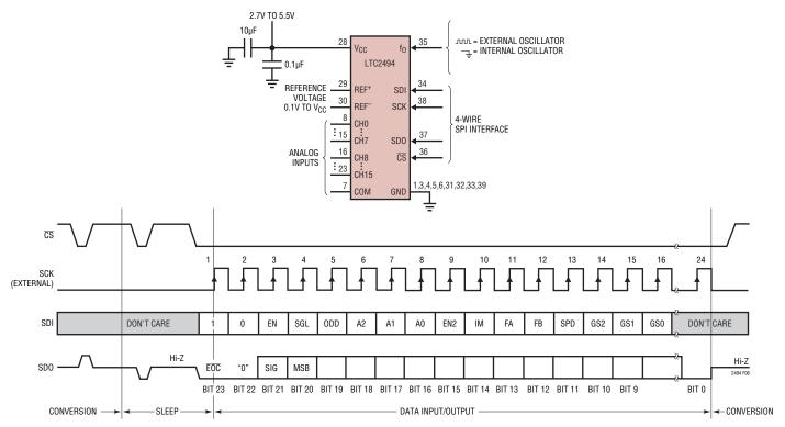
Figure 6. External Serial Clock, Single Cycle Operation
