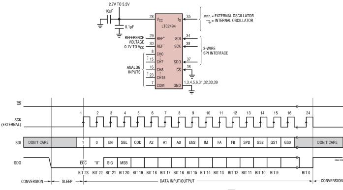
Figure 8. External Serial Clock, 3-Wire Operation ( $\overline{CS} = 0$ )
