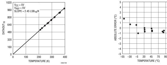
Figure 4. Internal PTAT Digital Output vs Temperature
