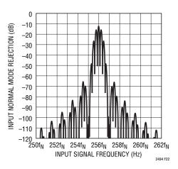
Figure 22. Input Normal Mode Rejection at  $f_S = 256 \bullet f_N$
