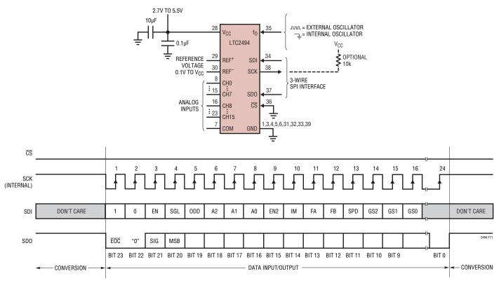
Figure 11. Internal Serial Clock, Continuous Operation
