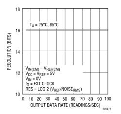
Figure 34. Resolution (Noise\_{RMS}  $\leq$  1LSB) vs Output Data Rate and Temperature
