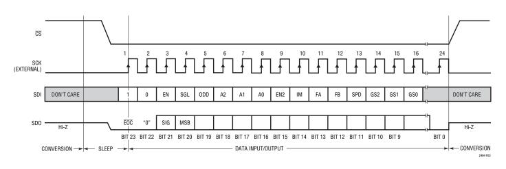
Figure 3. Channel Selection, Configuration Selection and Data Output Timing
