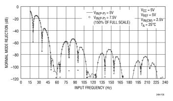
Figure 26. Measure Input Normal Mode Rejection vs Input Frequency with Input Perturbation of 150% (60Hz Notch)
