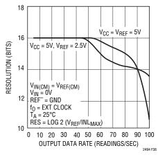
Figure 38. Resolution (INL<sub>MAX</sub>  $\leq$  1LSB) vs Output Data Rate and Reference Voltage
