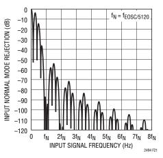
Figure 21. Input Normal Mode Rejection at DC
