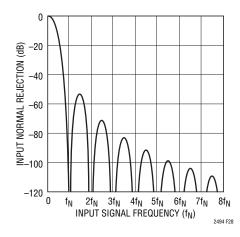
Figure 28. Input Normal Mode Rejection 2x Speed Mode
