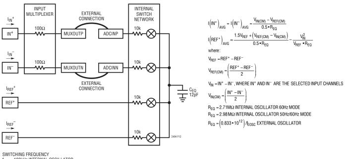
Figure 12. LTC2494 Equivalent Analog Input Circuit
