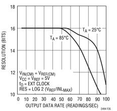
Figure 35. Resolution (INL<sub>MAX</sub>  $\leq$  1LSB) vs Output Data Rate and Temperature
