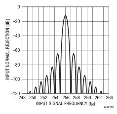
Figure 29. Input Normal Mode Rejection 2x Speed Mode
