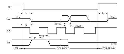
Timing Diagram Using Internal SCK (SCK HIGH with  $\overline{\text{CS}}{\downarrow})$
