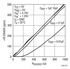
Figure 16. +FS Error vs R<sub>SOURCE</sub> at V<sub>REF</sub> (Large C<sub>REF</sub>)
