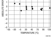
Figure 5. Absolute Temperature Error
