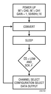
Figure 2. LTC2494 State Transition Diagram
