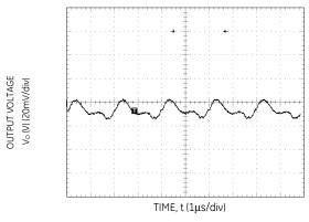
Figure 15. Typical output ripple and noise (V  $_{\mbox{\footnotesize IN}}=$  12V,  $I_{\mbox{\footnotesize o}}=$   $I_{\mbox{\footnotesize o},\mbox{\footnotesize max}}).$
