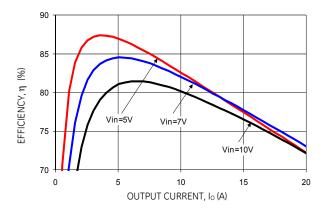
Figure 1. Converter Efficiency versus Output Current.
