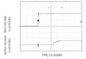
Figure 6. Typical Start-up Using Input Voltage ( $V_{IN} = 10V$ ,  $I_0 = I_0 = 0$ )
