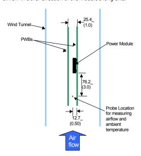
Figure 49. Thermal Test Setup.
