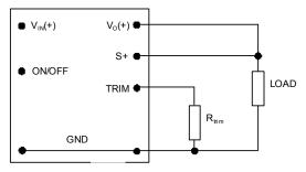
Figure 45. Circuit configuration for programming output voltage using an external resistor.
