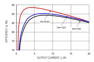
Figure 13. Converter Efficiency versus Output Current.
