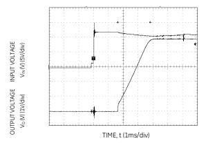
Figure 33. Typical Start-up Using On/Off Voltage ( $I_0 = I_{0,max}$ ).
