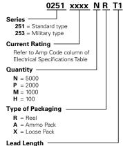
The default lead length for Ammo pack and Loose pack is now T1 for 251 series, and remains T3 for 253 series, therefore: T1 = 52.4mm (2.062"), 251 series only\* Blank = 52.4mm (2.062") for 251 series\* or 73mm (2.874") for 253 series\*\*
